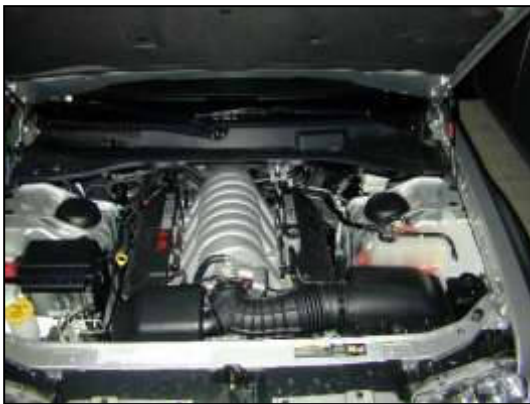
a. Stock air box system installed.
