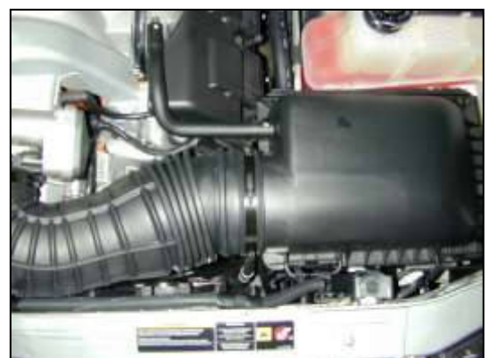
d. Loosen the inlet tube hose clamp. Remove the inlet tube.
