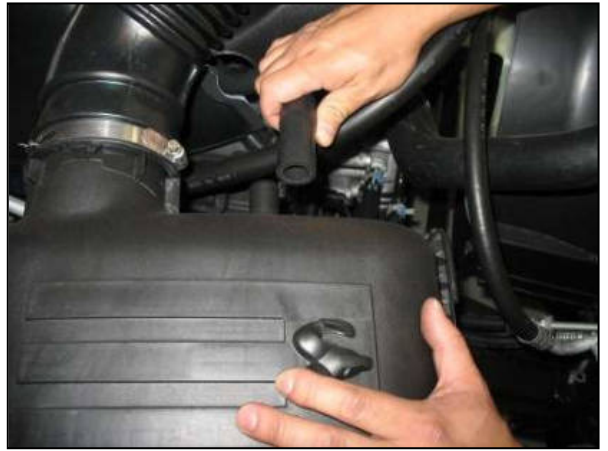
f. Disconnect the engine breather hose from the air box lid.
