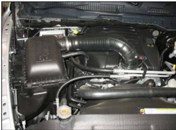
Factory air box system installed
