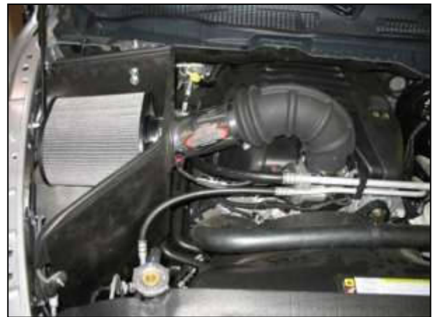
AEM® intake system installed
