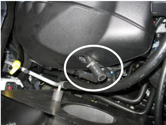
s. Re-install the factory engine cover, allowing the new breather hose to protrude from the access hole as shown. Place the second 1 1/4" hose clamp loosely on the end of the hose.
