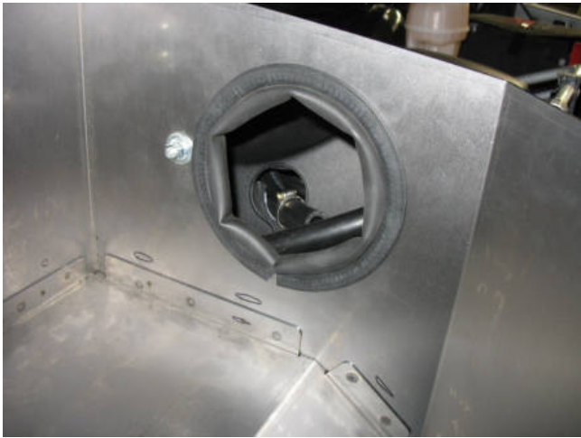
q. Install the medium section of the rubber sponge edge gasket in the large hole for the inlet tube as shown if you haven't done so previously.
