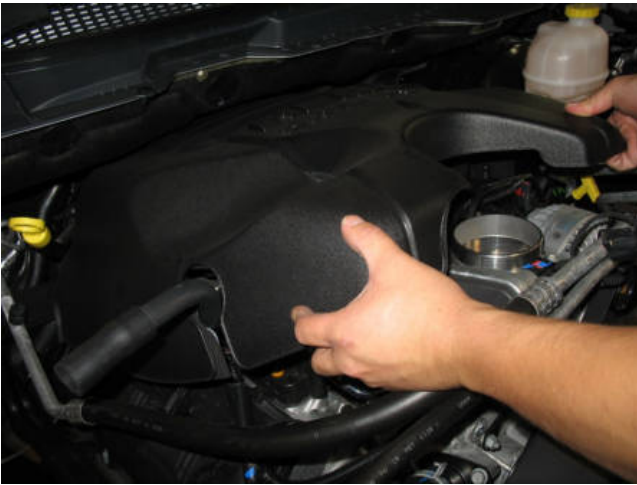
k. Remove the engine cover by lifting the front of the cover and then pulling forward.
