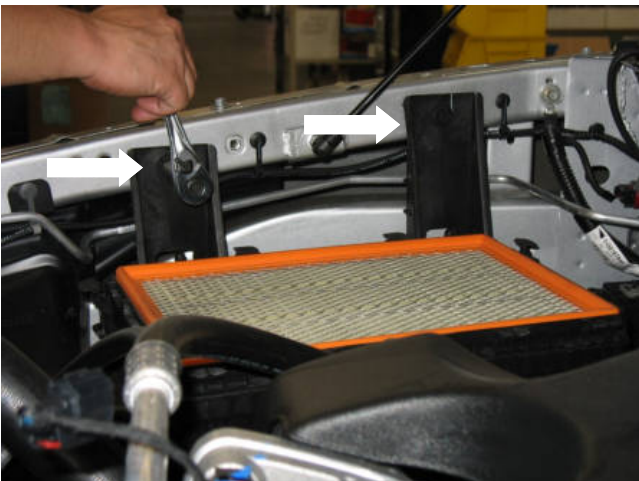
i. Remove the 2 bolts securing the air box base to the vehicle.
