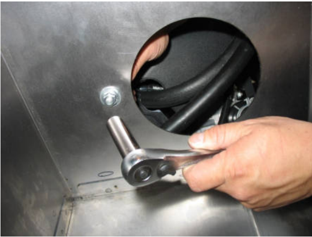
p. Use 1 M8 washer and 1 M8 nut inside the heat shield to secure the rubber mount.
