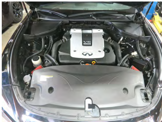
AEM INTAKE INSTALLED
