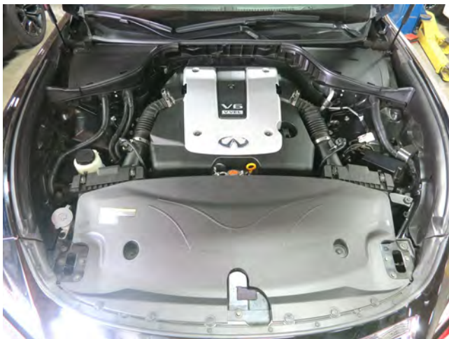
STOCK INTAKE INSTALLED
