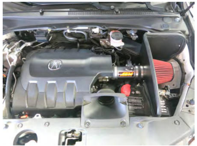
AEM INTAKE INSTALLED
