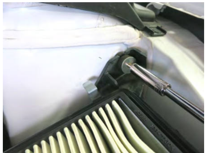
j. Remove the bolt securing the air box to the shock tower.
