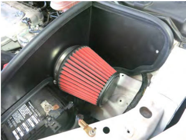
j. Install the AEM DryFlow air filter to the filter adapter with the provided hose clamp.
