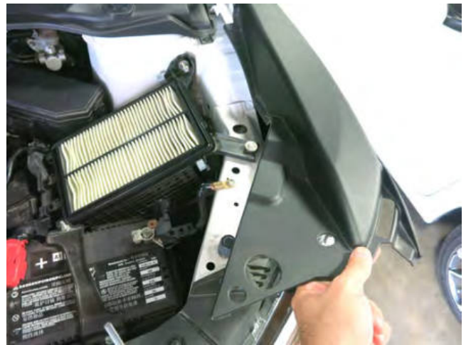
h. Remove the fender shrouding by pulling up gently to reveal the upper air box bolt.
