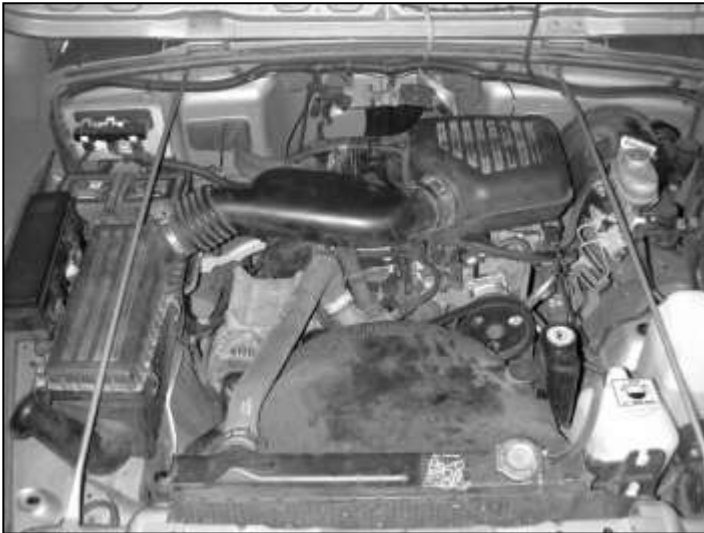
Factory air box system installed
