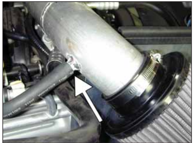
m. Reattach the breather hose to the nipple as shown.
