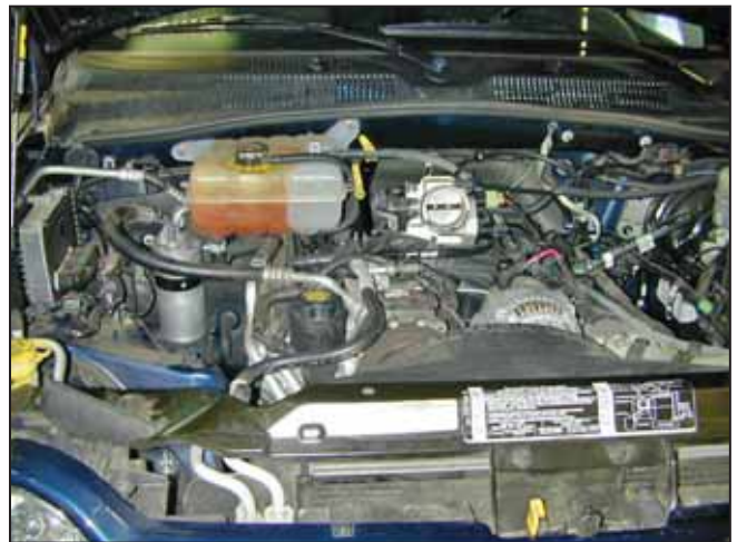
h. Stock air box system removed.
