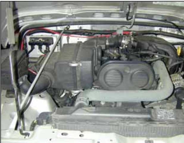
a. Factory air box system installed.
