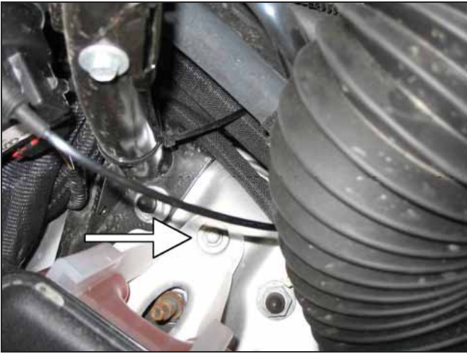
e. Loosen and remove the coolant reservoir mounting bolt.
