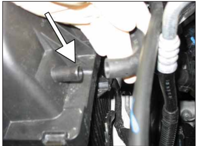
d. Disconnect the crankcase breather hose.
