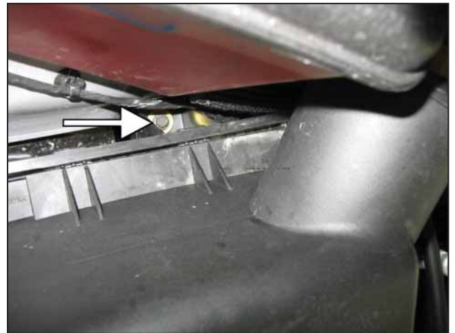
h. Loosen and remove the air box mounting bolt.
