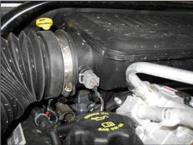
a. Disconnect the Inlet Air Temperature sensor.
