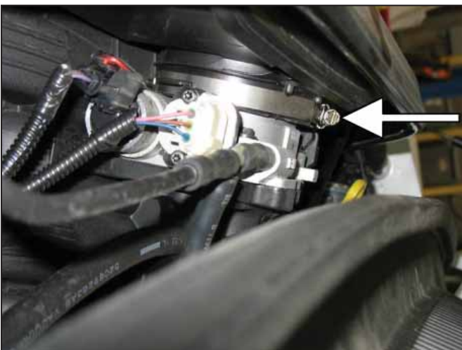
i. Loosen the throttle body hose clamp.
