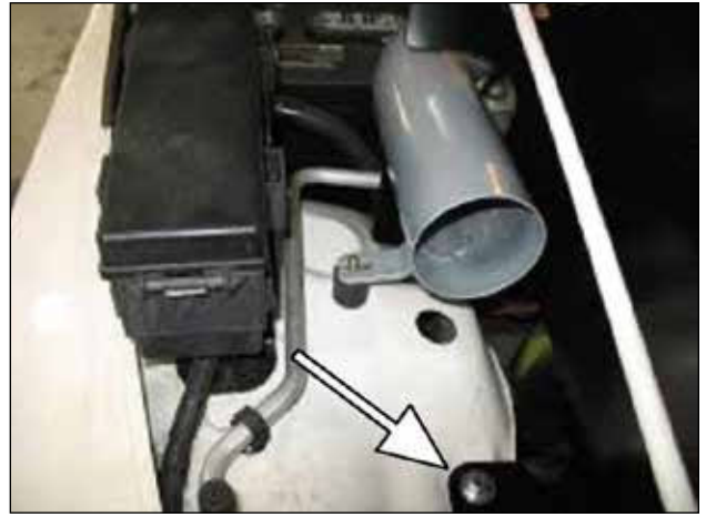
g. Align the intake pipe with the heat shield and rubber mount. After alignment is achieved, secure the heat shield with the supplied M8 bolt, washers and nut to the fender well of the vehicle.
