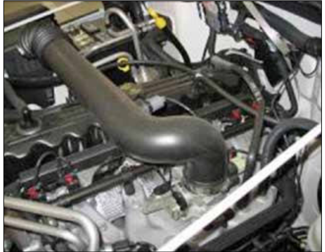
b. Loosen the hose clamp located at the throttle body.
