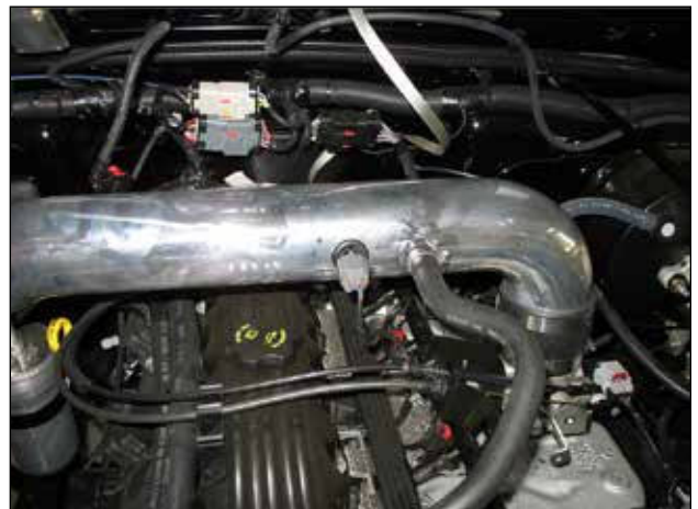
k. Attach the supplied breather hose to the intake pipe and the crank case ventilation nipple. Use supplied 1" hose clamps to secure the hose.
