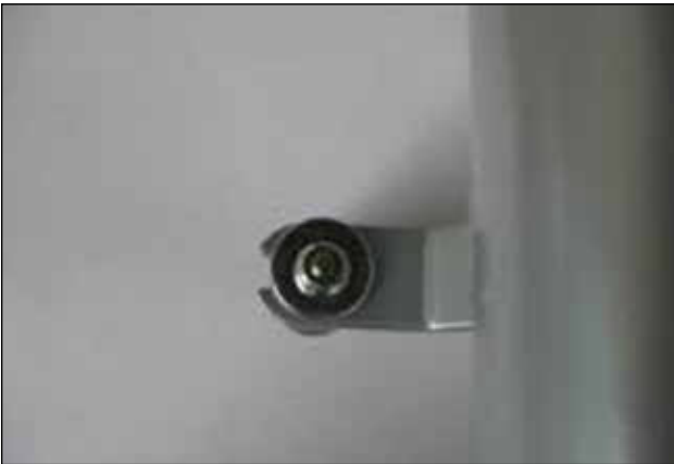
h. Secure the intake pipe to the rubber mount by using the supplied 6mm nut and washer.
