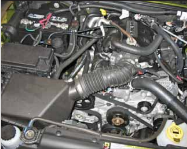
a. Factory air box configuration for Jeep Wrangler.
