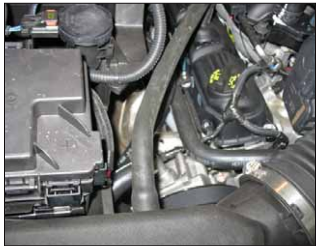
d. Remove the stock breather hose from the air box lid.
