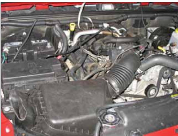
Factory air box system installed
