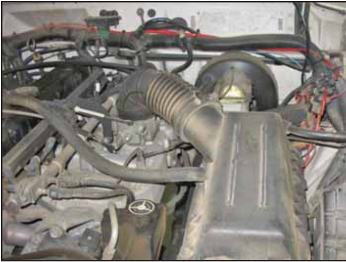
Factory air box system installed
