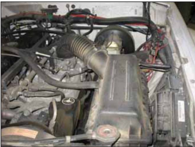
a. Factory air box system installed.
