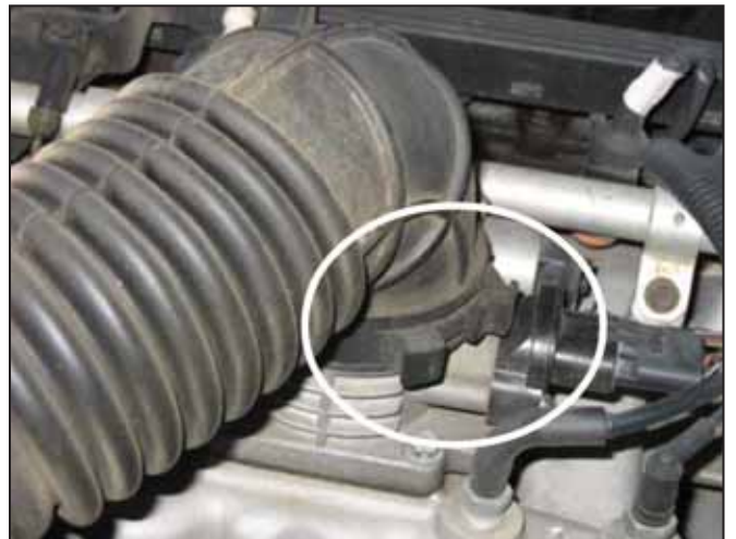
d. Loosen the hose clamp on the throttle body. This is done by simply pulling outward on the plastic hose clamp grips.
