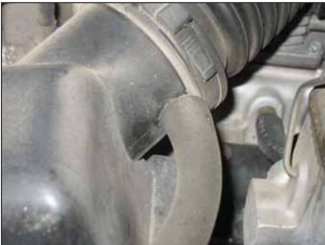
c. Remove the rubber hose connecting the hard plastic charcoal canister hose to the air filter housing.
