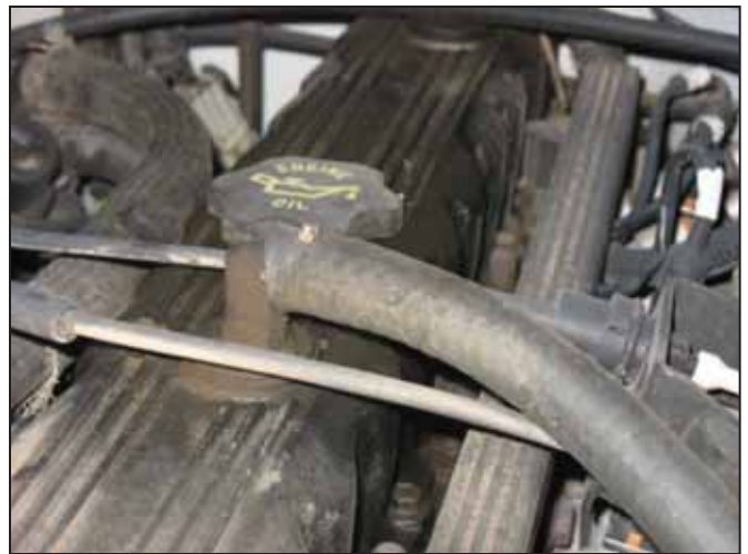
b. Remove the breather hose between the air filter housing and the valve cover.
