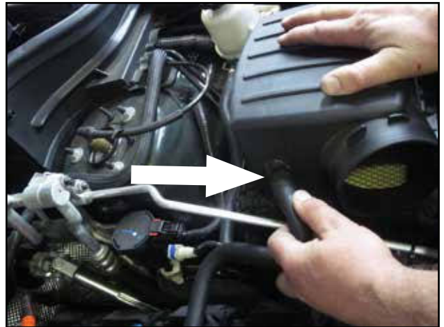
h. Detach the valve cover breather hose from the airbox.
