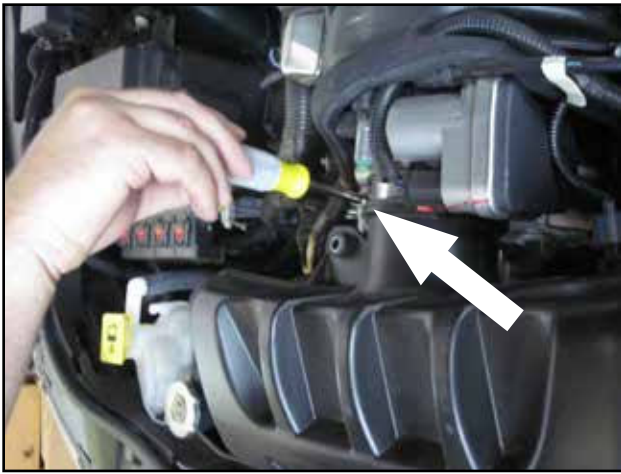
e. Loosen the hose clamp at the throttle body.
