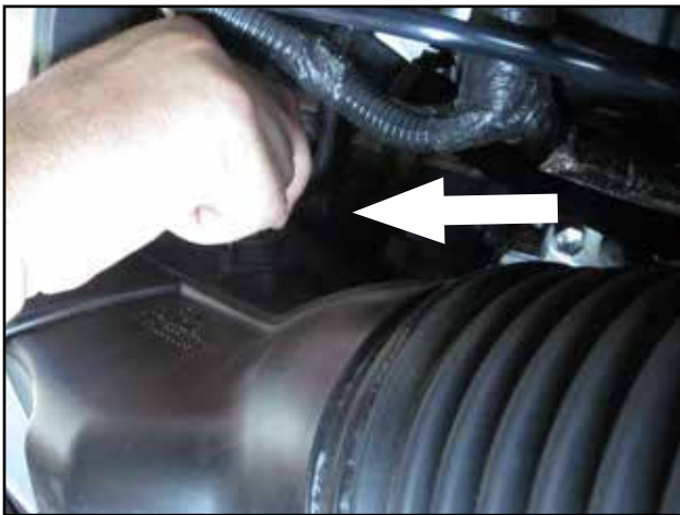
c. Disconnect the inlet air temperature (IAT) sensor wire harness from the sensor.
