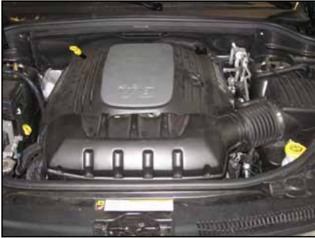
a. Your factory air intake system should look like this.
