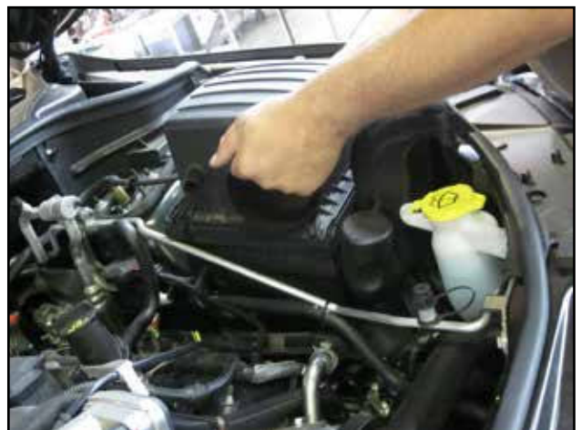
j. Lift and remove the air box from the engine bay.
