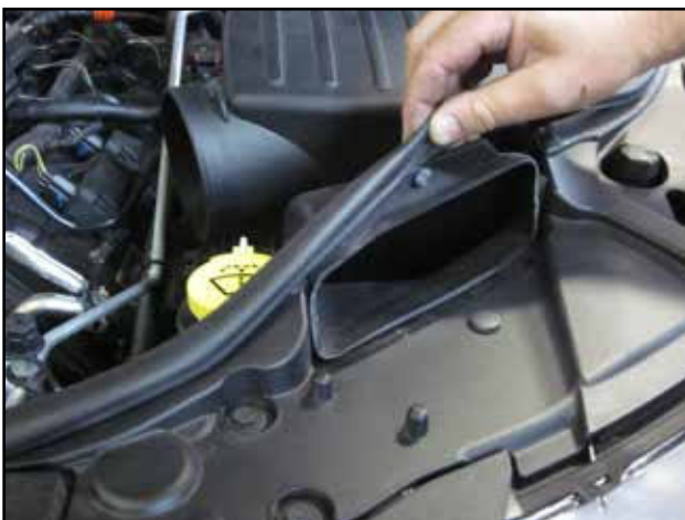
i. Detach the air inlet duct from the rubber edge trim.
