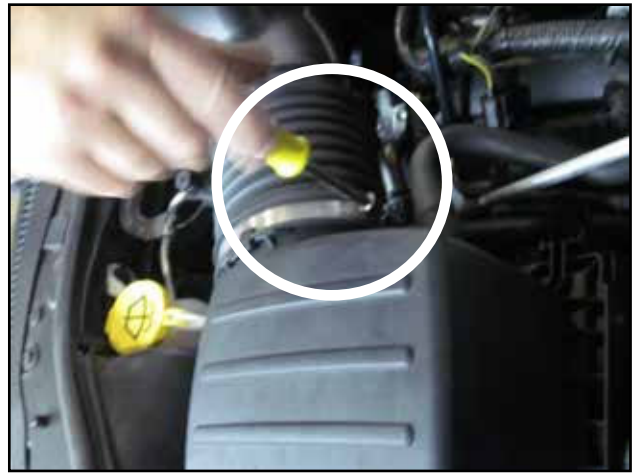
f. Loosen the hose clamp at the air box.
