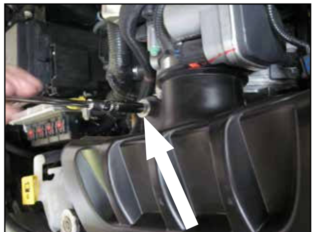
d. Loosen and remove the M6 air inlet chamber mounting bolt.
