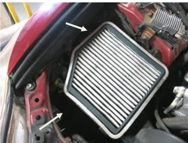
i. Remove the two bolts securing the air box base.
