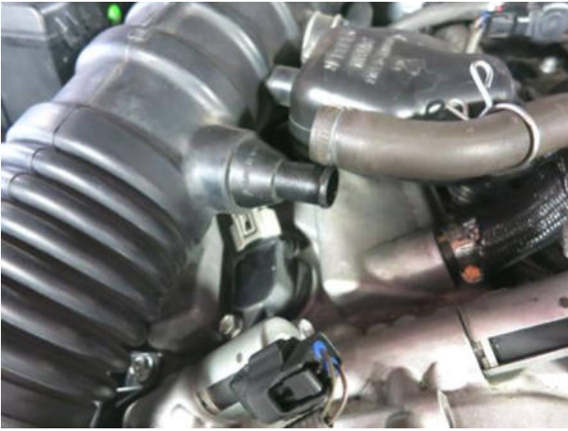
e. Disconnect the crankcase breather hose from the factory intake tract.
