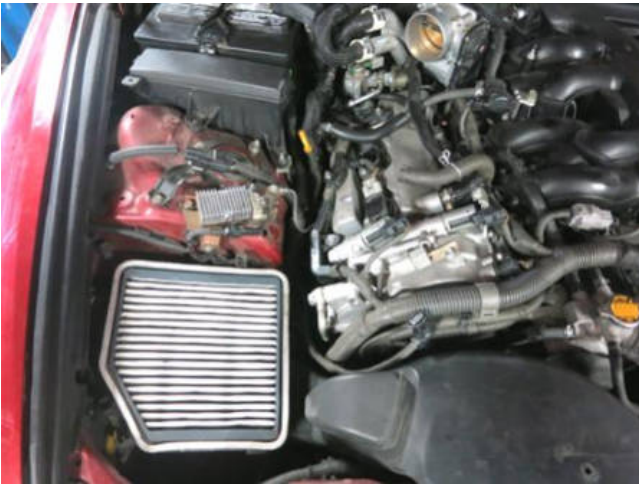
g. Unlatch the air box lid from its base and lift the air box lid and hose from the engine bay.
