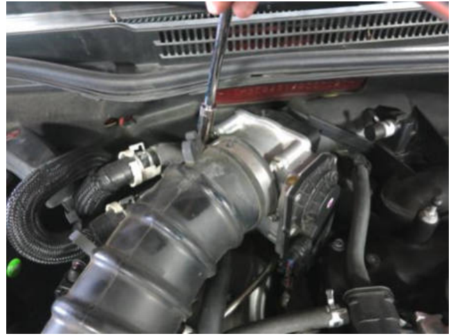
f. Loosen the hose clamp securing the intake tract to the throttle body.
