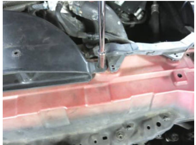
h. Remove the bolt securing the air scoop; it will be reused in step 3a.
