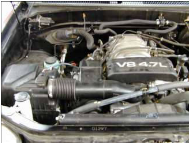
a. Stock air box system installed in vehicle.
