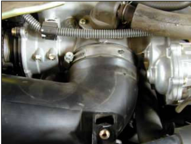
g. Loosen the hose clamp retaining the stock intake piping.
