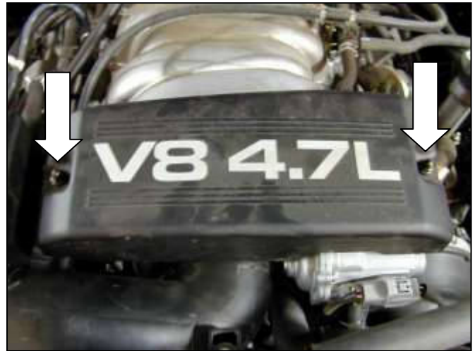
b. Remove the two nuts retaining the stock engine cover and remove.
