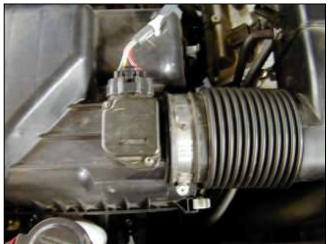
d. Remove the two screws retaining the MAF sensor and set them aside in a safe area. They will be installed with the AEM® intake system.
