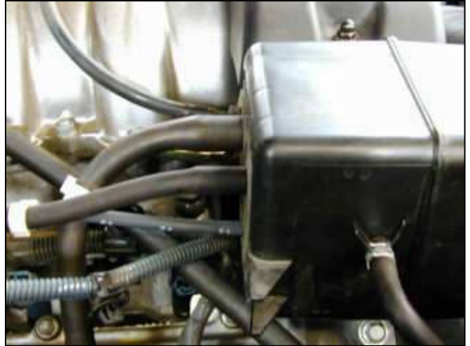
f. Remove the three hoses from the resonator chamber on the stock system. Some models have only two hoses and one vacuum cap to remove.
