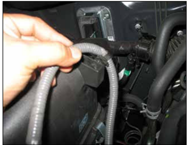
d. Release the zip tie from the airbox lid. Unplug the wire harness plug from the mass air flow sensor.
