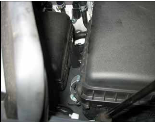
g . Unclip the third airbox clip.
