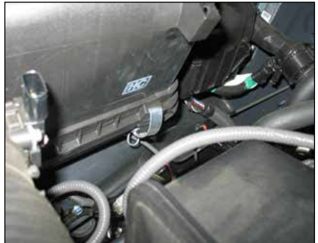
h. Unclip the fourth airbox clip.
