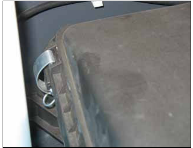
f. Unclip the second airbox clip.
