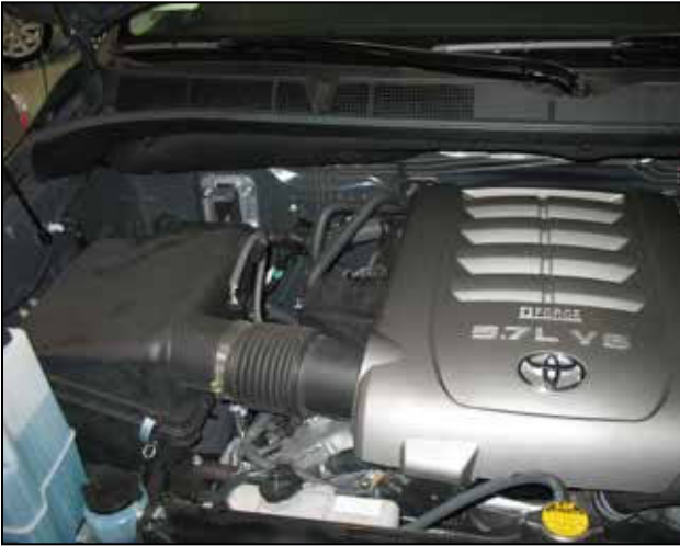
a. Factory airbox system installed.
