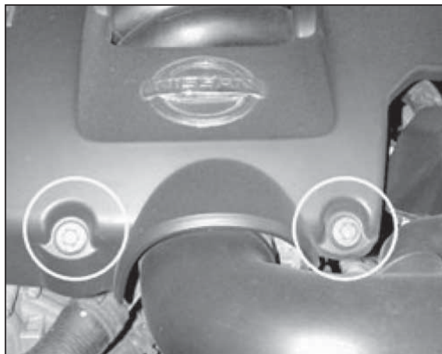
b. Remove the two screws securing the engine cover and remove the cover.
