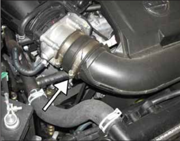
a. Loosen the hose clamp at the inlet tube side only.
