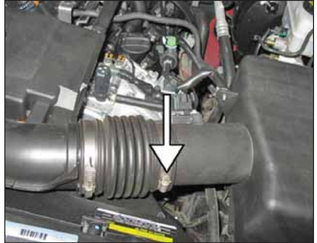
b. Loosen the hose clamp on the air box side.
