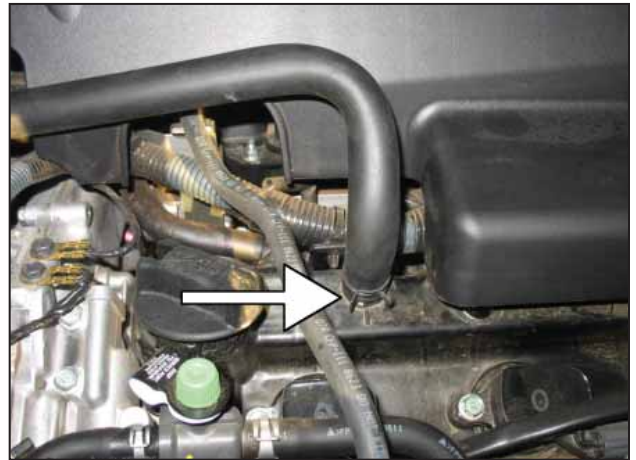
d. Remove the crank case breather tube from the valve cover; save the spring clamp for later use.
