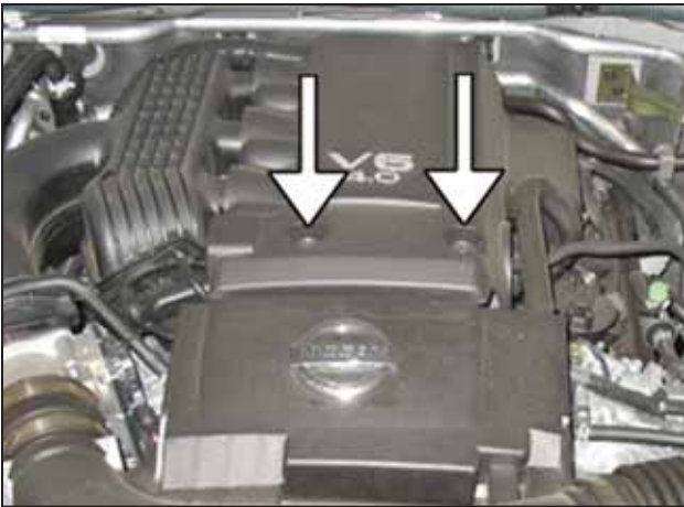
c. Loosen and remove the bolts to the engine cover; remove engine cover from vehicle.
