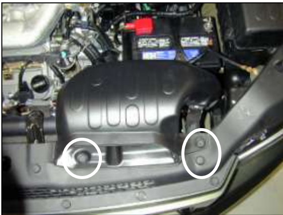
c. Remove the plastic intake air duct by removing the three plastic retaining clips. Be sure not to lose or damage any of these parts, they will be reused in installation.
