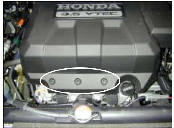
b. Remove the plastic intake air duct by removing the three plastic retaining clips. Be sure not to lose or damage any of these parts as they will be reinstalled.
