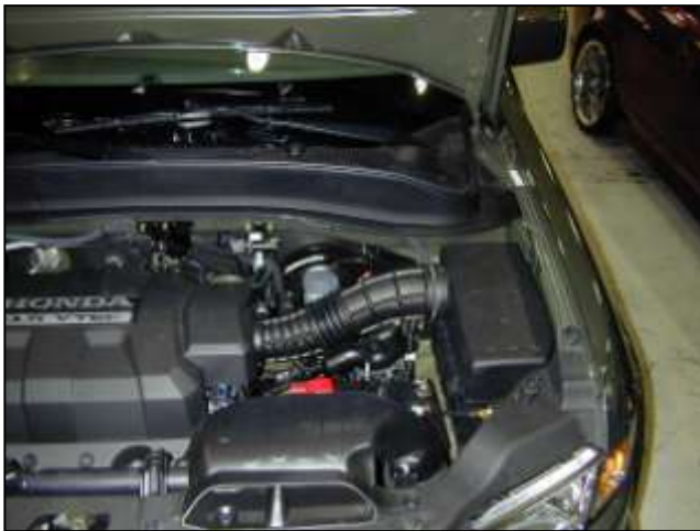
Stock air box system installed
