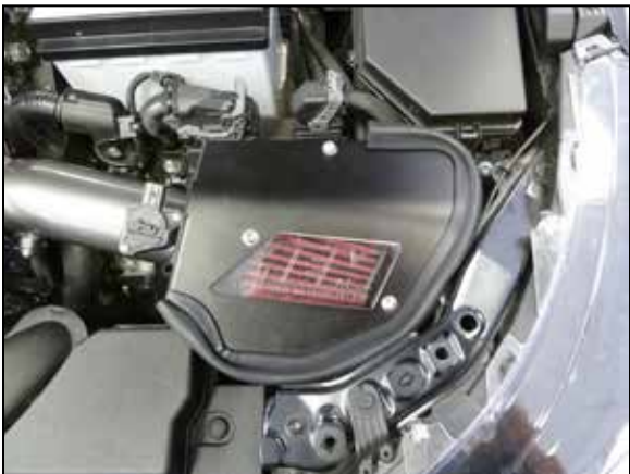
24. Install the heat shield lid and secure with the provided hardware.
