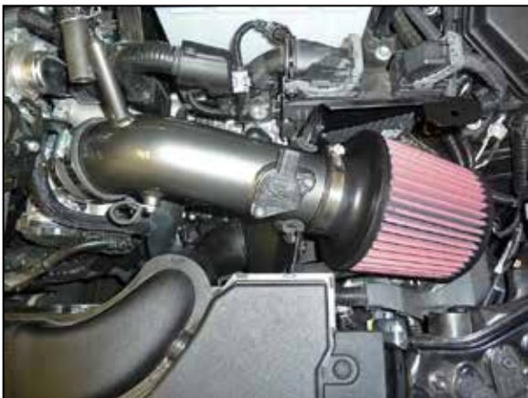
21. Install the intake tube assembly into the coupler at the throttle body and adjust for best fit.
