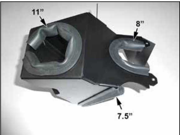
12. Install the 7.5", 8" and 11" edge trim onto the heat shield as shown.
