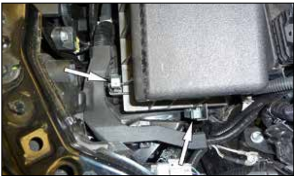
6. Release the two clips that secure the upper air filter housing and then remove the upper housing from the vehicle.
