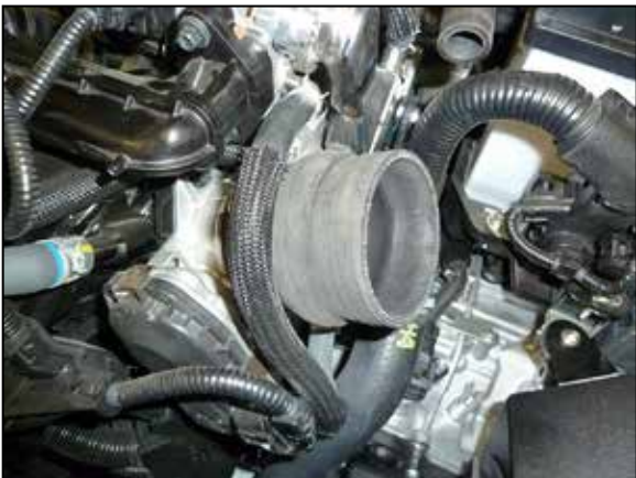
20. Install the provided coupler (084036) onto the throttle body and secure with the provided hose clamp.
