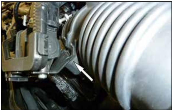
3. Disconnect the EVAP solenoid and bracket from the factory intake tube.
