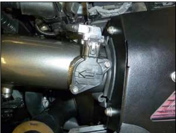
25. Reconnect the mass air electrical connection.
