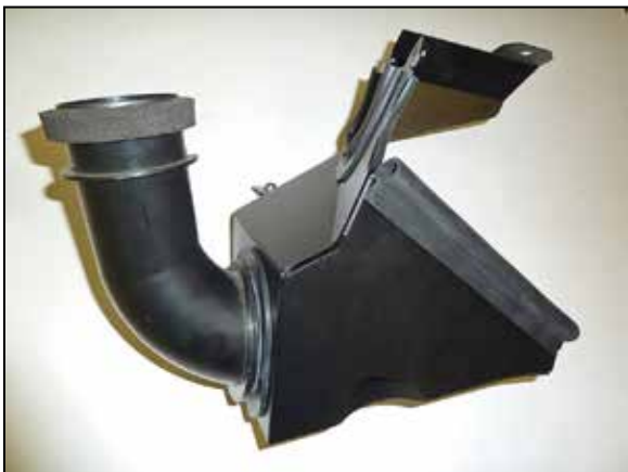
15. Install the fresh air intake duct into the hole of the heat shield as shown.
