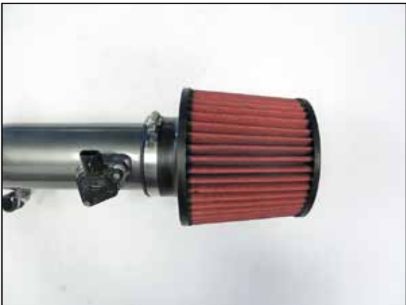
19. Install the AEM® air filter onto the intake tube and secure with the provided hardware.
