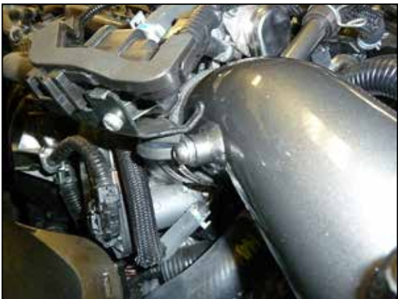
23. Insert the EVAP solenoid bracket into the adel clamp attached to the intake tube.
