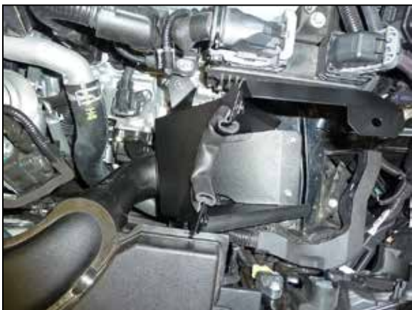
16. Install the heat shield assembly and align the fresh air intake duct. Secure the assembly with the provided hardware.
