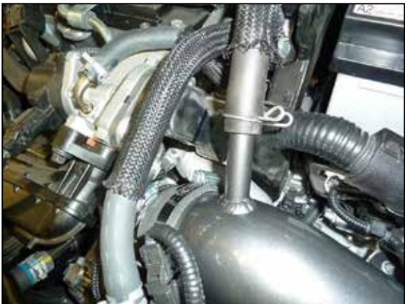
22. Connect the PCV hose to the AEM® intake tube and secure with the factory spring clamp.
