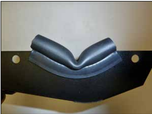
11. Install the 3.5" edge trim onto the bottom of the heat shield lid as shown.
