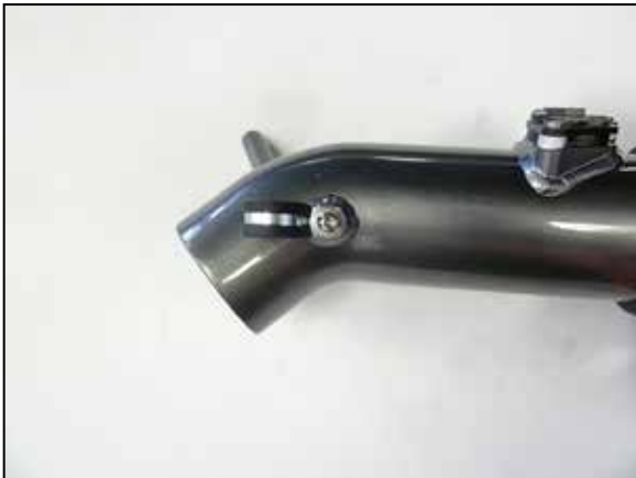
18. Install the provided loop clamp onto the AEM® intake tube and secure with the provided hardware.
