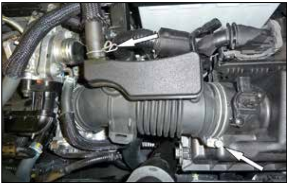
5. Remove the PCV hose from the factory intake tube and then loosen the hose clamp that secures the intake hose to the air filter housing and then remove it from the vehicle.
