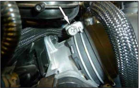
4. Loosen the hose clamp that secures the intake tube to the throttle body.
