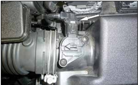
2. Disconnect the mass air sensor electrical connection.
