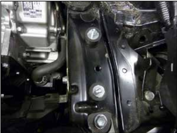
8. Install the two provided rubber mounted studs into the frame at the factory air filter housing mounting locations.
