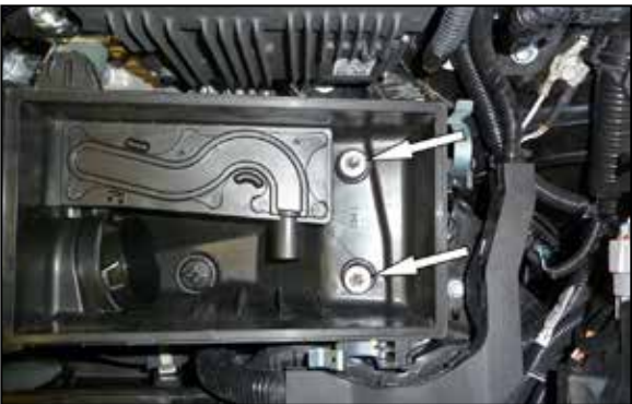
7. Remove the two bolts that secure the lower air filter housing and then remove the housing from the vehicle.
