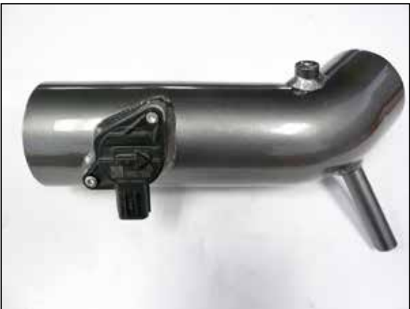
17. Remove the mass air sensor from the factory air filter housing and then install it into the AEM® intake tube and secure with the hardware provided.
