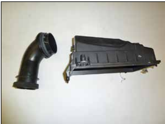
14. Remove the factory fresh air intake duct from the factory air filter housing.
