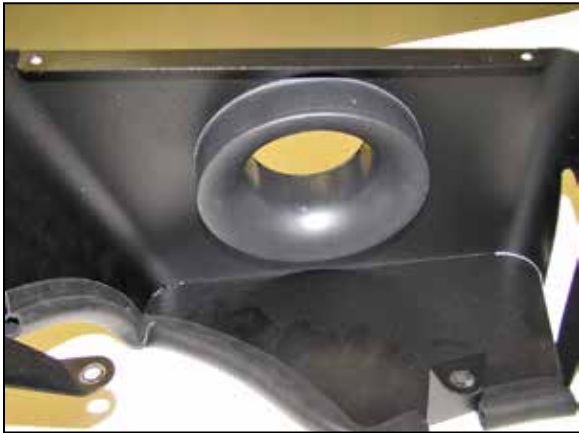
10. Install the radius filter adapter into the heat shield and secure with the provided hardware.
