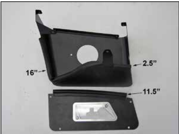
9. Install the edge trim onto the heat shield and lid as shown.
