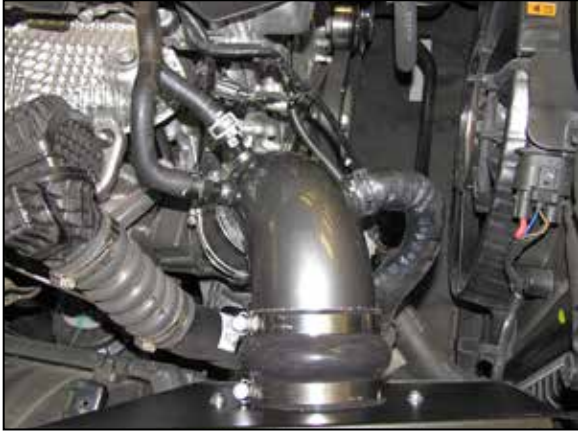
15. Install the AEM® intake tube into the couplers and adjust for best fit and secure with the provided hose clamps. Connect the vent lines and BOV hose and secure with the factory spring clamps.
