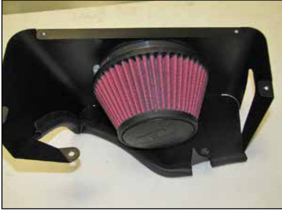
11. Install the AEM® air filter onto the filter adapter and secure with the provided hose clamp.
