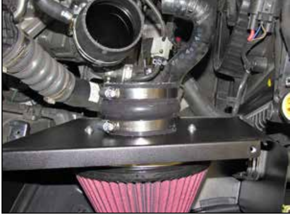
13. Install the provided hump coupler onto the filter adapter and secure with the hose clamp.
