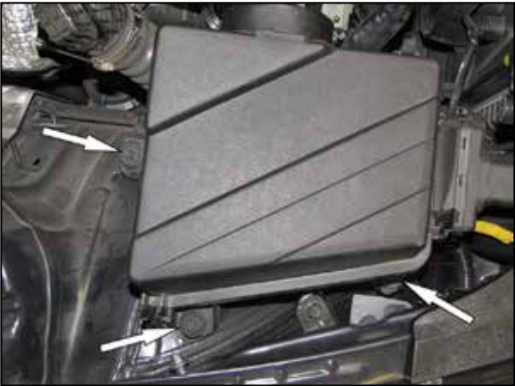
5. Remove the three bolts that secure the air filter housing and then remove the housing from the vehicle. NOTE: AEM recommends that customers do not discard factory air intake.
