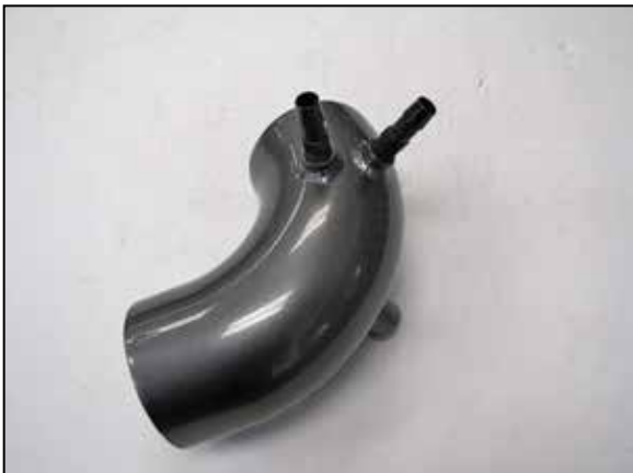
14. Install the vent fittings into the AEM® intake tube as shown. NOTE: Plastic NPT fittings are easy to cross thread. Install the vent fitting “hand” tight, then turn it two complete turns with a wrench.
