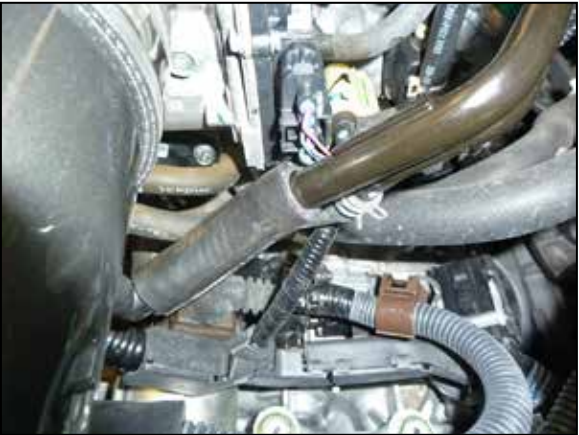
16. Connect the factory CCV hardline to the CCV hose attached to the intake tube.
