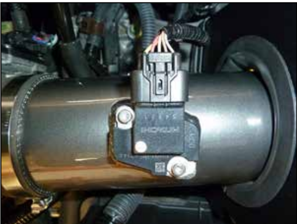
17. Reconnect the mass air sensor electrical connection.
