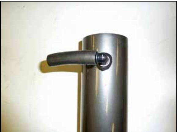
13. Install the 90° vent fitting and provided CCV hose into the AEM® intake tube as shown. NOTE: Plastic NPT fittings are easy to cross thread. Install the vent fitting "hand" tight, then turn it two complete turns with a wrench.
