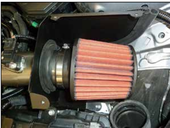
18. Install the AEM® air filter and secure with the provided hose clamp.
