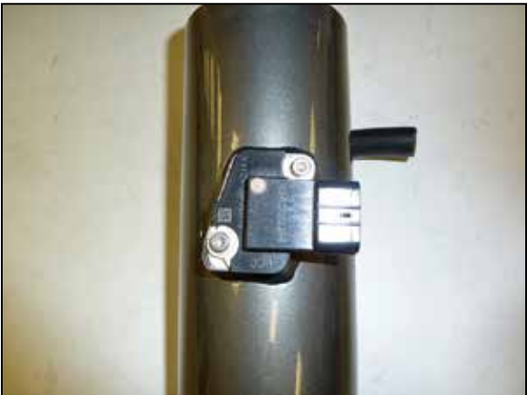
14. Remove the mass air sensor from the factory air filter housing and install it into the AEM® intake tube and secure with the provided hardware.
