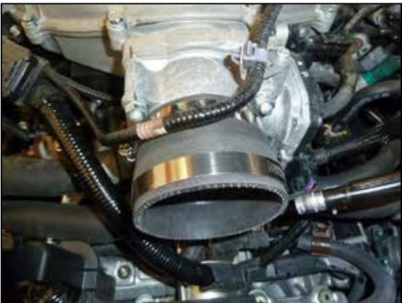
12. Install the provided coupler (084091) onto the throttle body and secure with the provided hose clamp.
