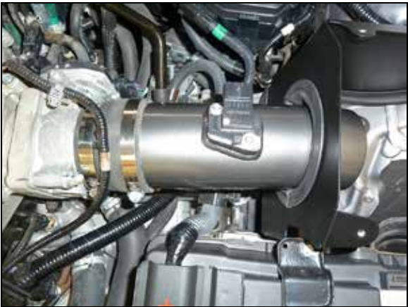
15. Install the intake tube assembly through the heat shield and then into the coupler at the throttle body. Adjust the tube for best fit and then secure with the provided hose clamp.
