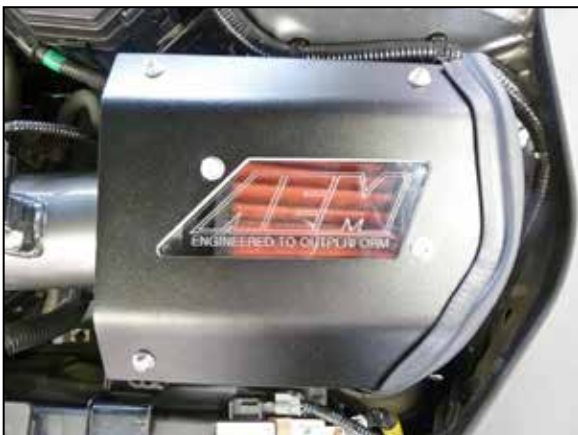
21. Install the cover assembly onto the heat shield and secure with the provided hardware.
