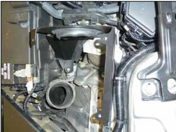
11. Install the heat shield assembly into the vehicle and secure with the provided hardware.
