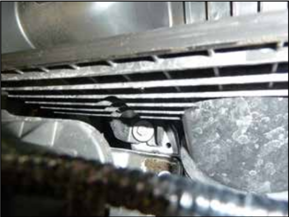
8. Remove the front air filter housing mounting bolt and remove the lower air filter housing from the vehicle. It may be necessary to move or remove the battery hold down to gain access to the bolt. NOTE: AEM recommends that customers do not discard factory air intake.
