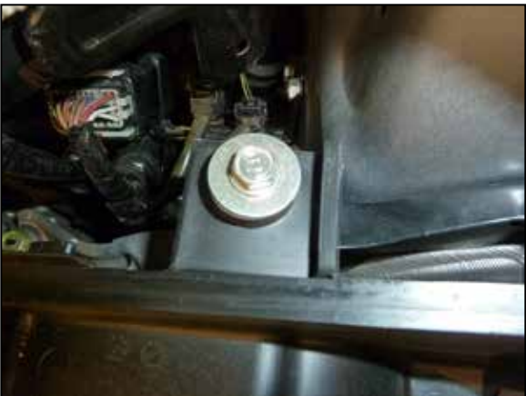
7. Remove the rear air filter housing mounting bolt.
