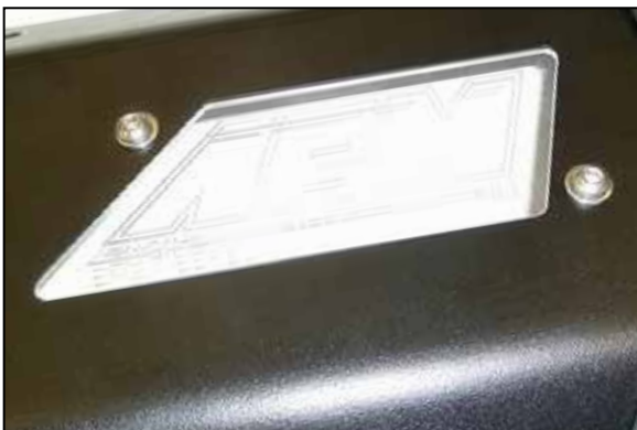
19. Install the AEM® window into the heat shield cover and secure with the provided hardware.
