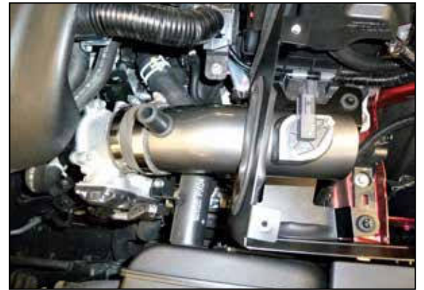
14. Install the K&N intake tube assembly through the heat shield and into the coupler at the throttle body, adjust the tube for best fit and then secure with the provided hose clamp.
