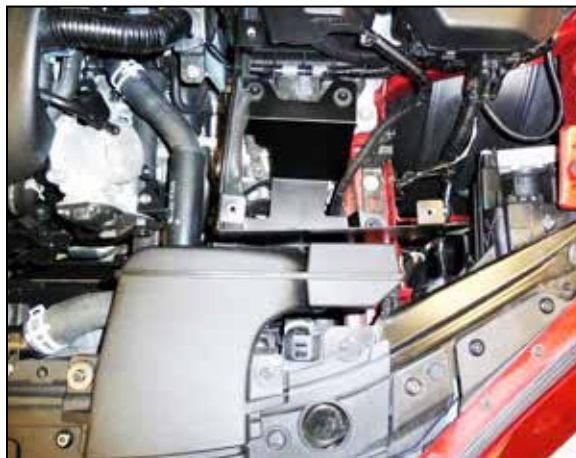
11. Install the heat shield assembly into the vehicle so the grommets engage the mounting studs. Secure the fresh air duct to the core support with the factory bolts.
