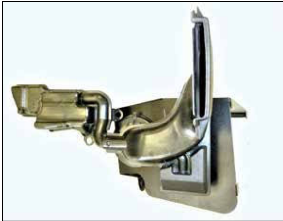
10. Install the factory fresh air intake duct into the heat shield assembly as shown.
