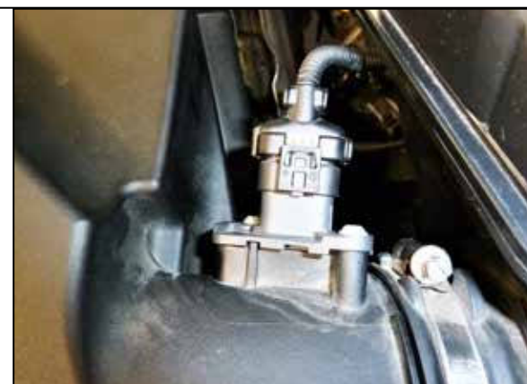
3. Release the locking tab and then disconnect the mass air sensor electrical connection.
