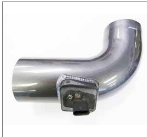
11. Remove the mass air sensor from the factory air filter housing and install it into the AEM intake tube using the provided hardware.
