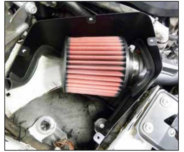
13. Install the air filter onto the intake tube and secure with the provided hose clamp. Adjust the tube and filter assembly for best fit and then secure the intake tube with the provided hose clamp.
