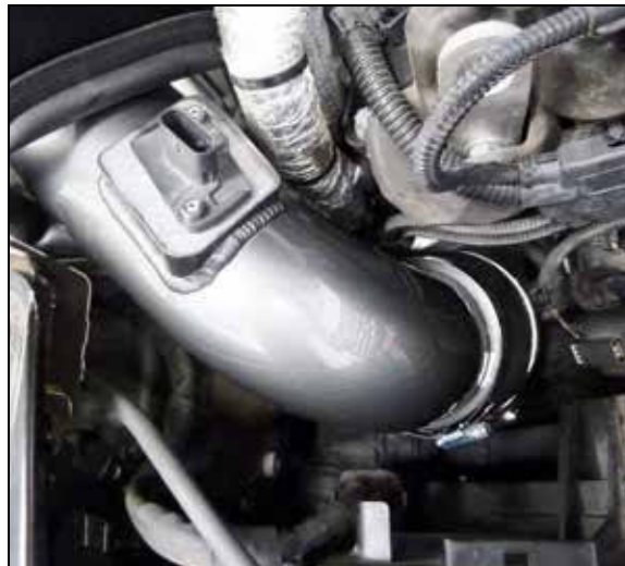
12. Install the intake tube through the heat shield and into the coupler. Do not secure the intake tube at this time.
