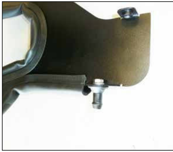
9. Install the heat shield mounting post onto the heat shield using the provided hardware.
