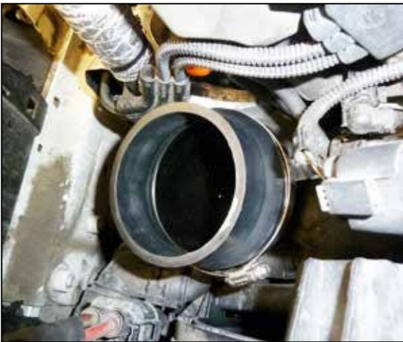
6. Install the provided coupler onto the turbo inlet and secure with the provided hose clamp.
