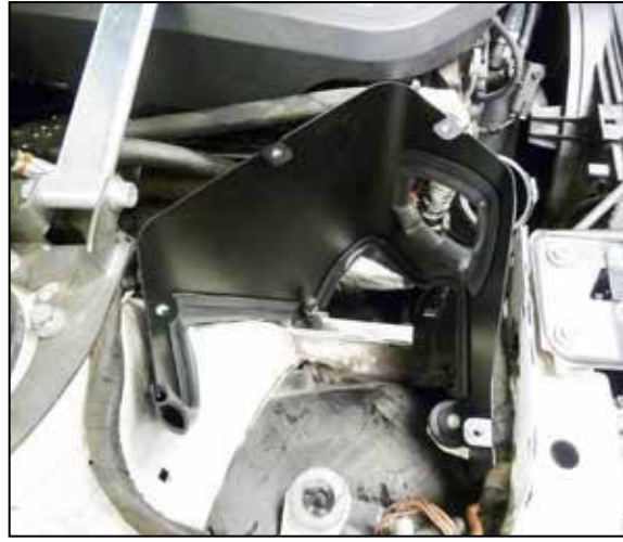
10. Install the heat shield into the vehicle so the mounting stud inserts into the factory grommet and onto the factory stud and secure with the provided hardware.
