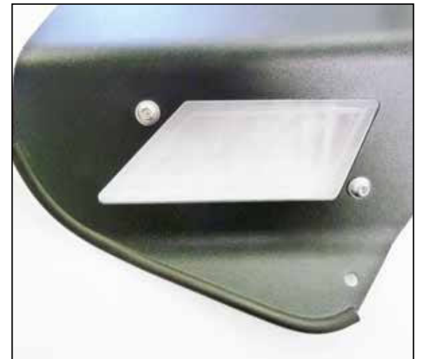
15. Install the provided edge trim onto the heat shield lid as shown using the provided super glue. Install the AEM window into the lid using the provided hardware and spacer.
