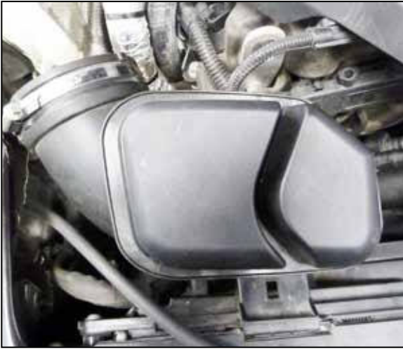
5. Loosen the hose clamp that secures the factory intake tube and then remove the tube from the vehicle.
