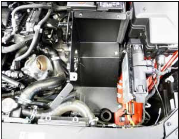
11. Install the heat shield assembly onto the rubber mounted studs and secure with the provided hardware.
