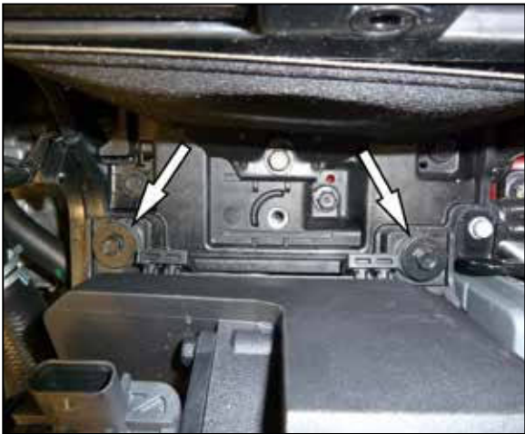
7. Remove the two rear air filter housing mounting bolts and then remove the complete intake assembly.
