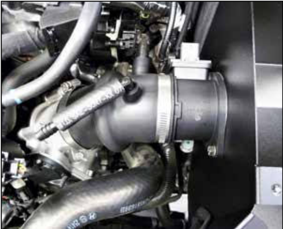
14. Install the hose/maf housing assembly onto the throttle body and into the heat shield. Adjust the maf housing so the holes line up and secure with the provided hardware. Adjust the hose for best fit and then secure with the provided hose clamps.
