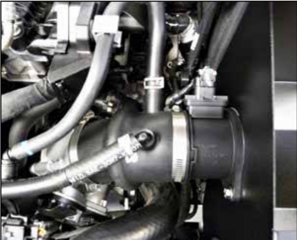
15. Reconnect the vent lines and secure with the factory spring clamps. Reconnect the mass air sensor electrical connection.
