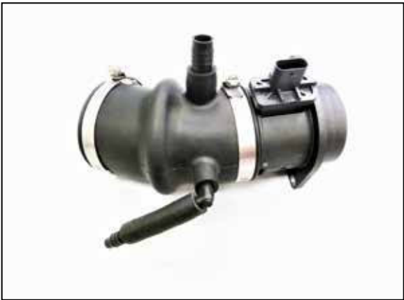
13. Install the factory mass air sensor into the AEM hose as shown but don't tighten the clamp.
