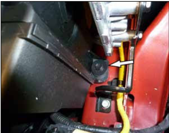
6. Remove the lower air filter housing retaining bolt.
