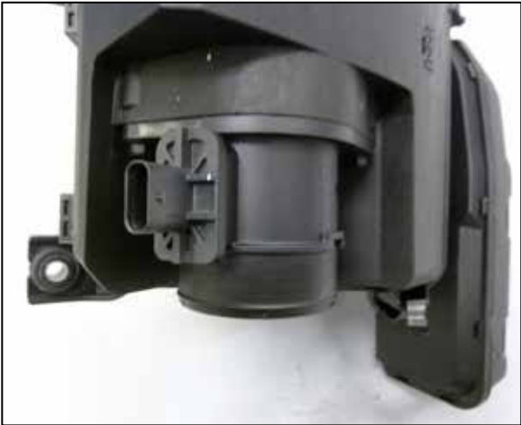
8. Remove the two bolts that secure the mass air sensor to the upper air filter housing and then remove the sensor from the housing.
