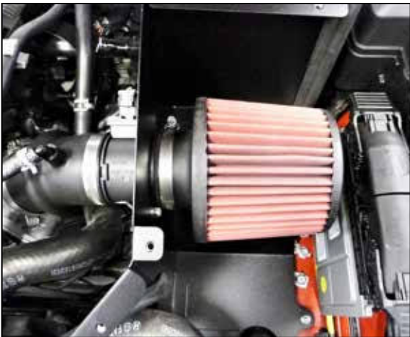
16. Install the AEM air filter onto the mass air sensor and secure with the provided hose clamp.
