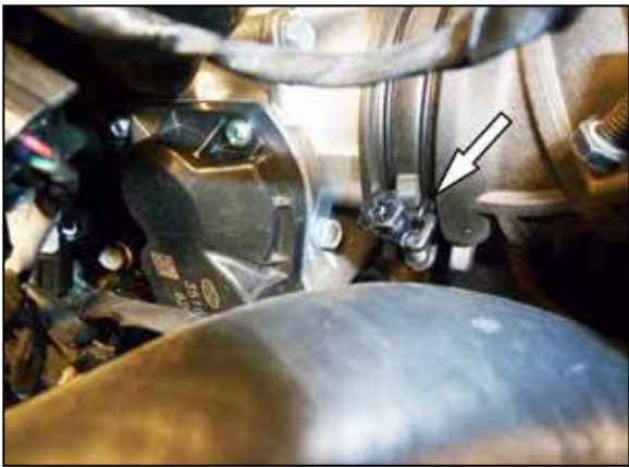
4. Loosen the hose clamp that secures the factory intake tube to the throttle body.
