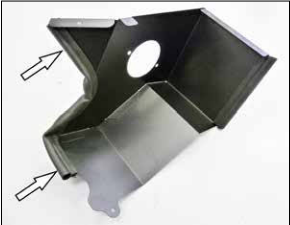
10. Cut a 7" long section of the edge trim and then install the edge trim onto the heat shield as shown trimming off access.
