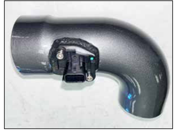
12. Remove the mass air sensor from the factory air filter housing and install it into the AEM intake tube and secure with the provided hardware.
