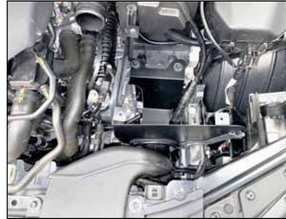
10. Install the heat shield assembly onto the mounting posts and secure the fresh air intake duct with the factory hardware.
