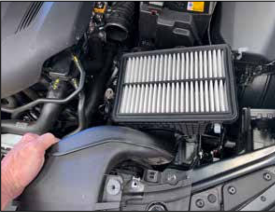
4. Pull up the lower air filter housing to dislodge it from the mounting grommets and remove it from the vehicle.
