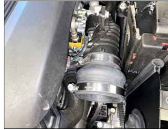
11. Install the provided hump coupler and secure with the provided hose clamp.
