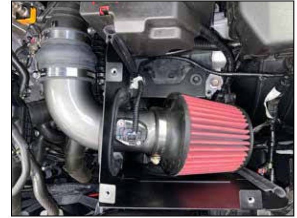
14. Install the air filter onto the intake tube and secure with the provided hose clamp.
