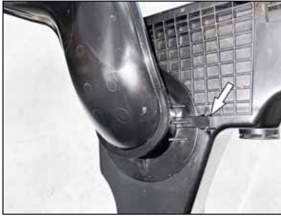
8. Release the tab that locks the fresh air duct to the lower air filter housing then rotate the fresh air duct counterclockwise and remove it from the housing.
