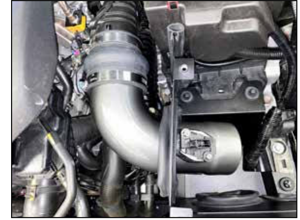
13. Install the AEM intake tube through the heat shield and into the coupler. Secure the coupler with the provided hose clamp.
