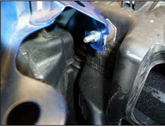
4. Remove the nut that secures the air filter housing vibration damper to the core support.
