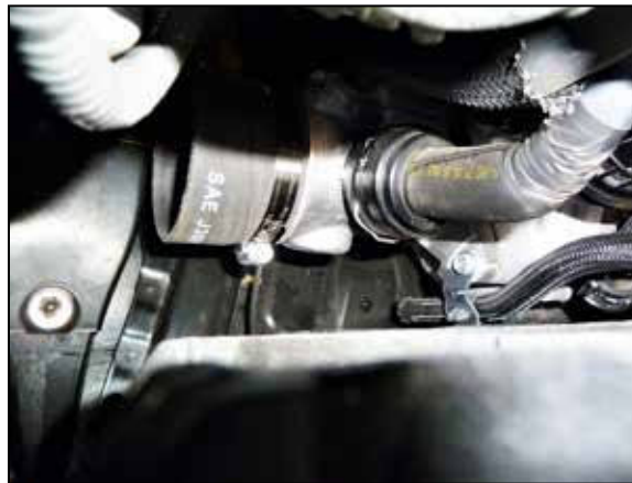
11. Install the provided coupler onto the turbo inlet and secure with the provided hose clamp.
