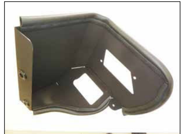
16. Install the provided edge trim onto the heat shield as shown. Some trimming of the edge trim will be necessary.
