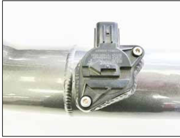
8. Remove the MAF sensor from the factory housing and install it into the AEM intake tube using the provided hardware.
