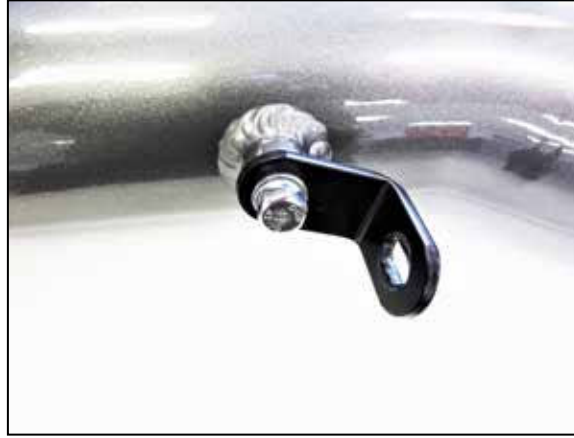
9. Install the provided "L" bracket onto the AEM intake tube using the provided hardware, do not completely tighten at this time.
