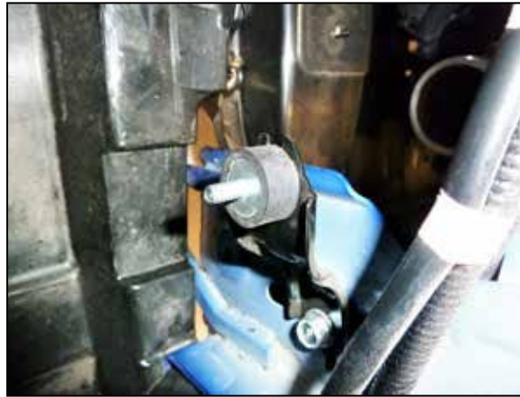
10. Remove the lower factory vibration damper and replace with the damper provided. Secure with the factory nut.
