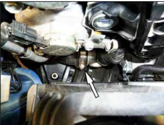
7. Loosen the hose clamp that secures the turbo inlet tube to the turbo and then remove the tube from the vehicle.
