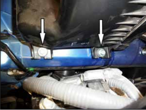
5. Remove the two bolts that secure the air filter housing to the inner fender.
