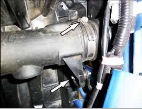
6. Remove the nut that secures the lower portion of the factory intake tube to the vibration damper and then loosen the hose clamp securing the intake tube to the turbo inlet tube. Remove the factory intake tube from the vehicle.
