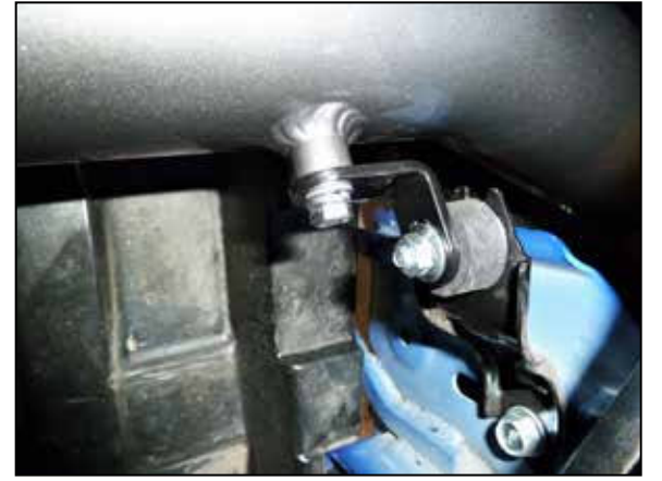
13. Position the "L" bracket onto the vibration damper, align the tube for best fit and then secure the hardware and hose clamp.
