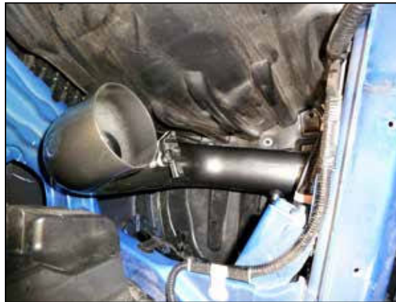
12. Position the AEM intake tube down thru the frame and into the coupler at the turbo.
