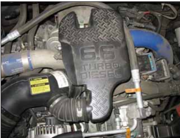
c. Lift up on the intake resonator to pop it off the mount. Loosen the hose clamps on both ends of the inlet tube.
