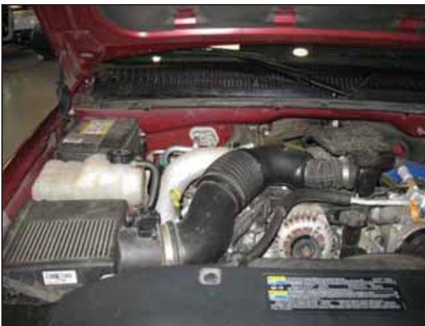
Factory air box system installed
