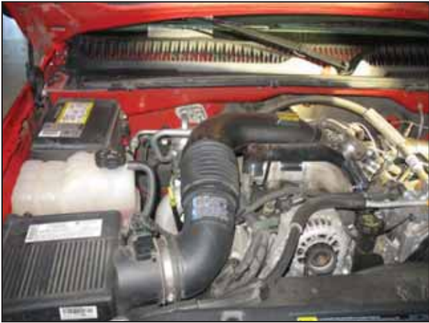
a. Factory air box system installed.
