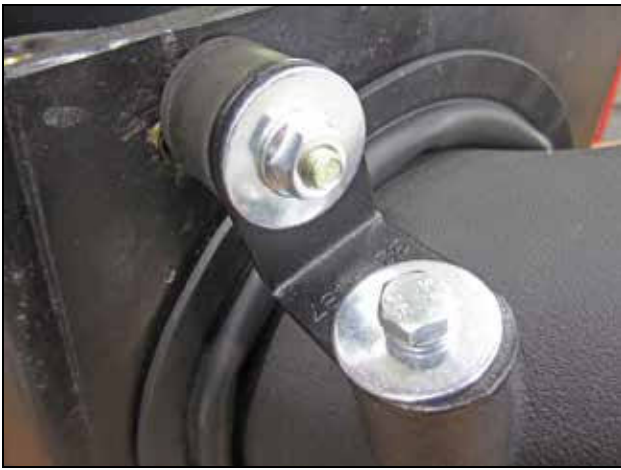
r. Install one flat washer, one split washer, and one M6 hex bolt through the "L" bracket slot and into the mounting boss in the lower intake tube. Tighten the bolt and the hex nut with a 10mm socket.
