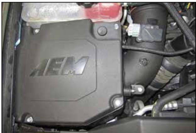
w. Install the air box lid onto the air box as shown using the M6 hex/flange bolts provided. Start all 4 bolts by hand first and then tighten them with a 10mm socket to seal the air box.
