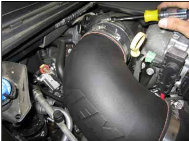
u. Fully seat the silicone hose at the engine intake port and tighten the hose clamp. The intake tube and filter installation is now complete. You are now ready to seal the air box.
