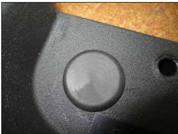
v. Install the plug into the 0.75" hole in the corner of the air box lid as shown.
