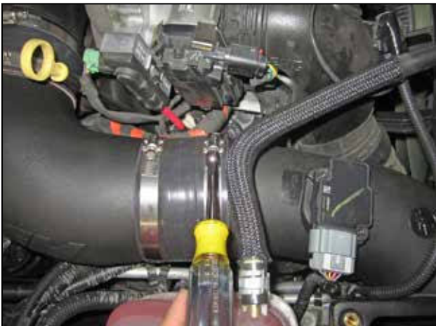
t. Tighten the hose clamp at the silicone hose connecting the lower intake tube to the intake elbow.
