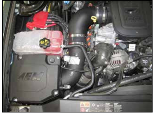
AEM® intake system installed.
