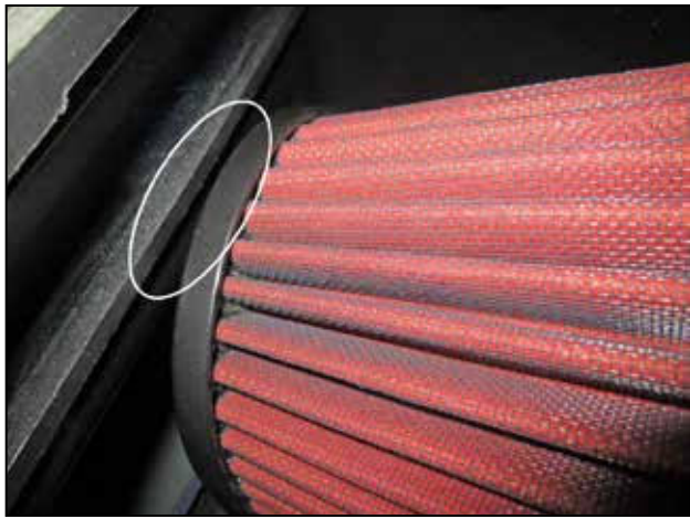
s. Rotate the lower intake tube and filter assembly until the edge of the filter cap lines up with the top edge of the air box opening near the fender as shown.
