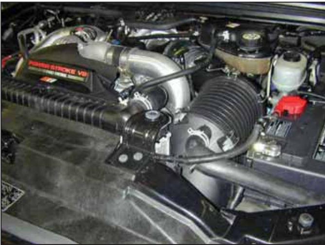
Factory air box system installed
