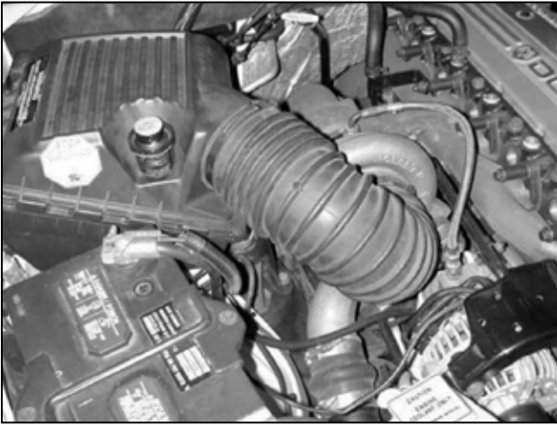
a. Factory air box system
