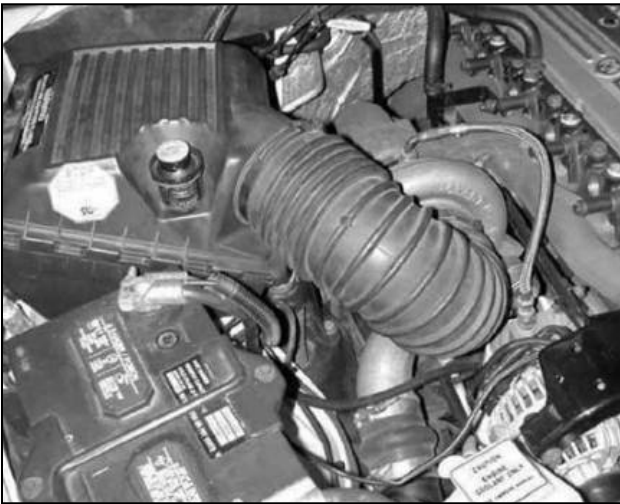
Factory air box installed
