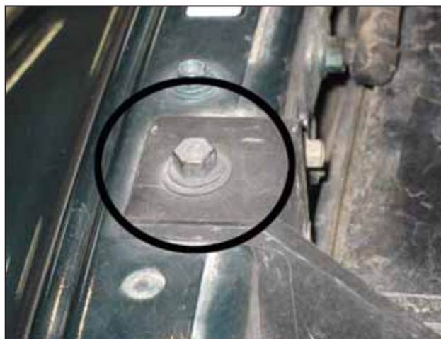
d. Remove the grommets from the plastic battery tray. Remove the bolt securing the battery tray to the fender.
