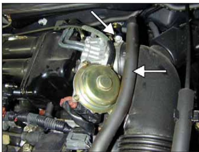
b. Pull breather hose off of valve cover. Loosen the upper and lower hose clamps on the stock inlet tube.
