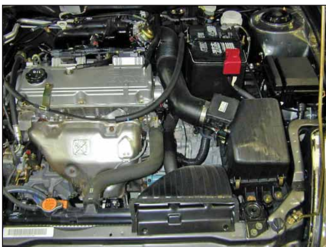
a. Factory air box system installed.
