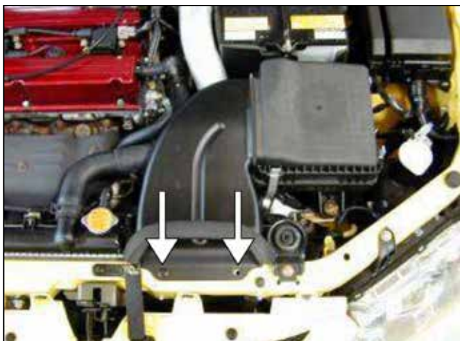
a. Push in the inner circle on the clips to remove them. Remove both clips. Remove inlet duct to air box.
