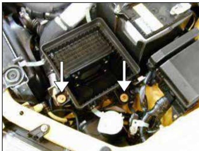
d. Remove the filter element. Remove the bolts holding down the bottom portion of the air box.
