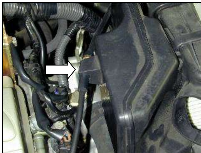
d. Unclip the throttle cable from the side of the air filter housing.
