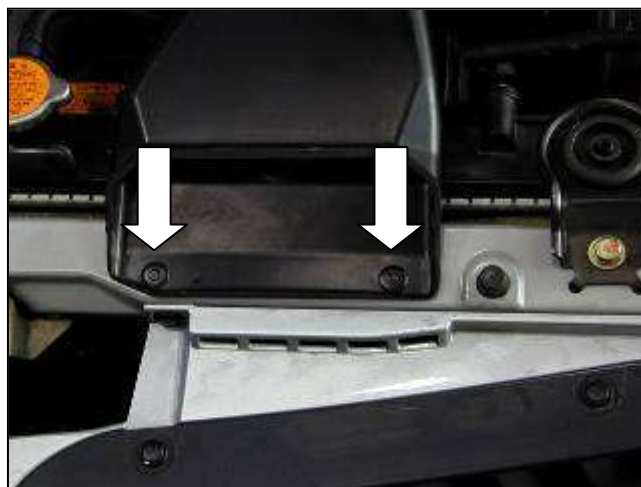
b. Remove the plastic inlet duct from the front of the engine bay by removing the plastic clips and then pulling the duct straight forward. To remove the clips, use a pointed tool and push in the middle of the clips.
