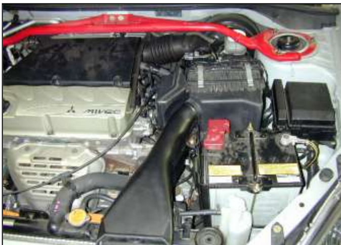
Factory air box system installed
