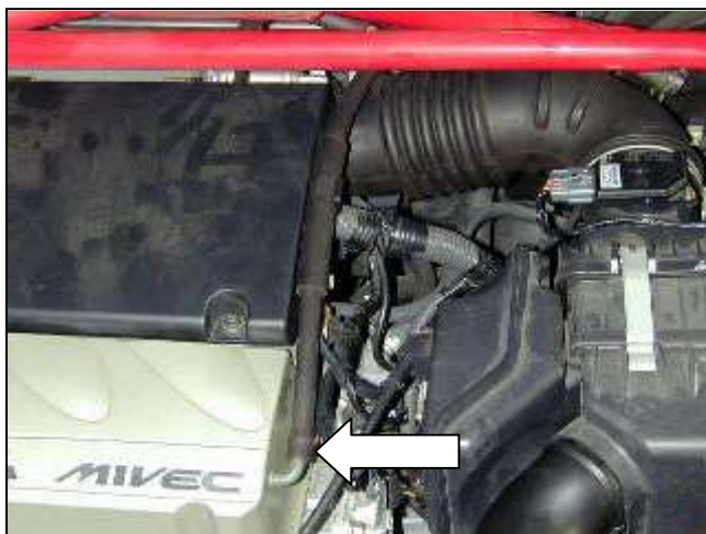
c. Remove the breather hose from the valve cover.
