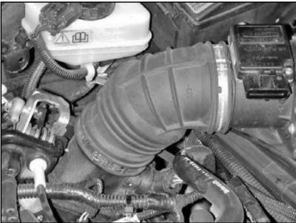
c. Remove the clamp securing the primary intake pipe to the throttle body.
