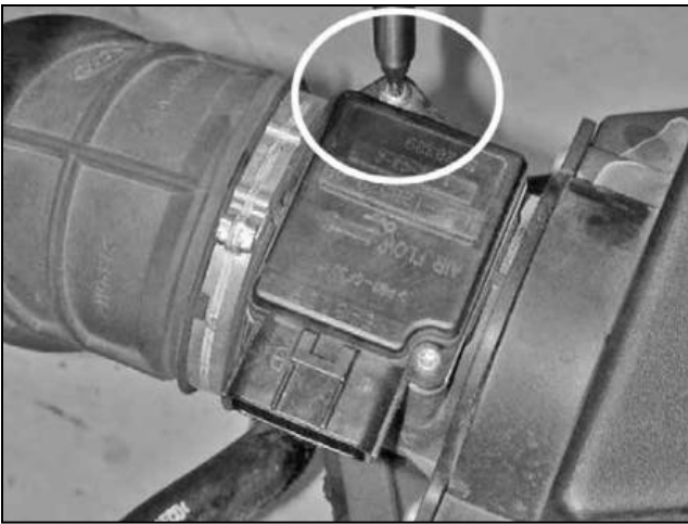
g. Remove the MAF sensor from the stock intake system.
