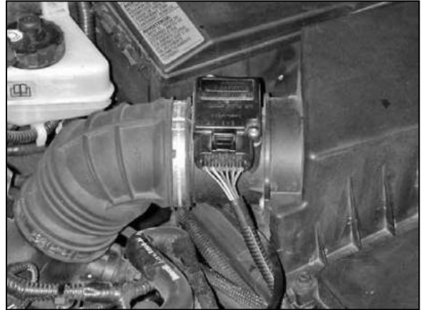
b. Remove the wiring harness from the MAF sensor.
