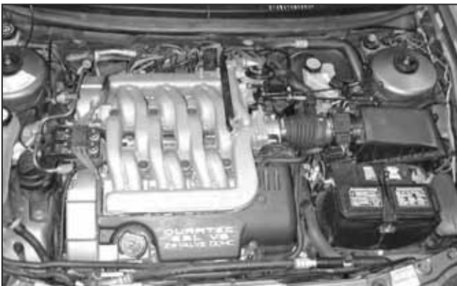
Stock air box system installed
