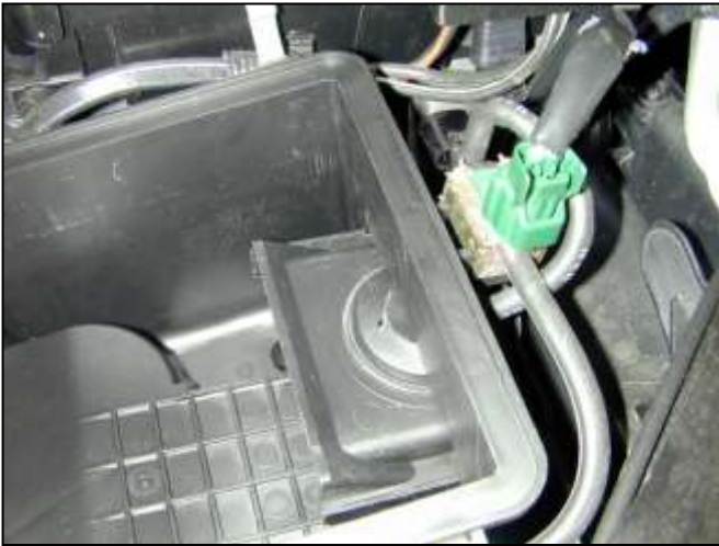
e. Unplug green connector on the vacuum solenoid.
