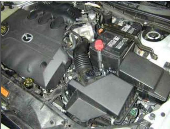
a. Stock air box system installed.
