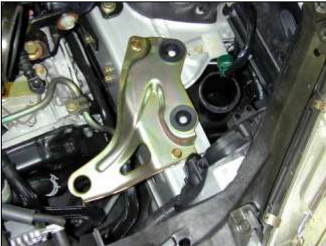
g. Pull the air box up and out of the engine bay. Remove the two bolts holding down the air box bracket and remove the bracket from the vehicle.
