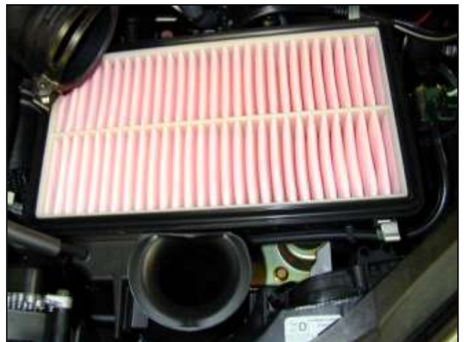
d. Remove the air filter from the lower air box.
