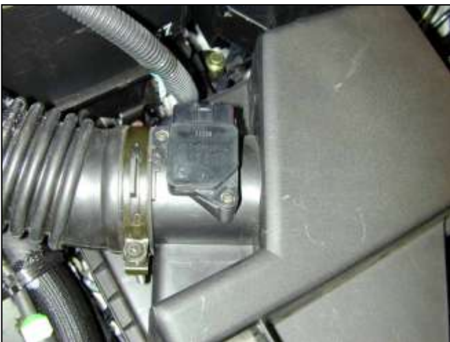
c. Release all clips and remove upper air box from vehicle. Loosen the two screws securing the MAF sensor and remove it from the air box.
