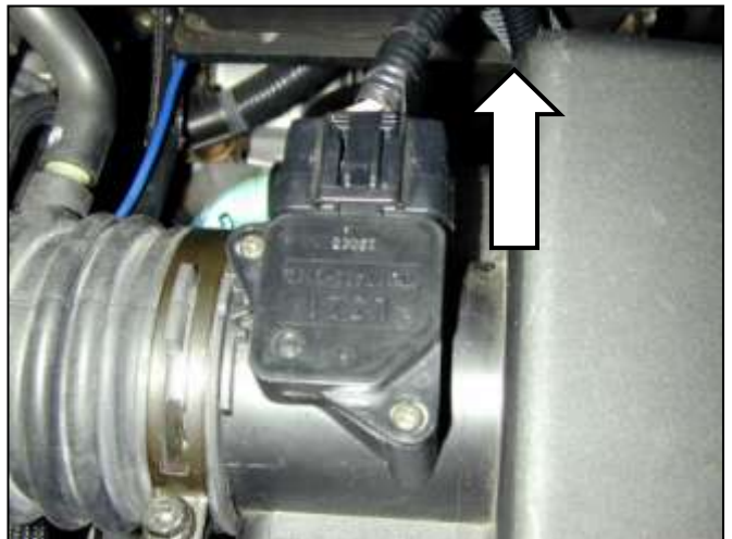
d. Unplug the mass air flow (MAF) sensor. Remove MAF sensor from air box.
