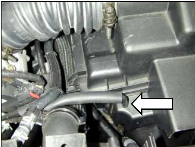
c. Pull the vacuum hose off of the air box nipple.
