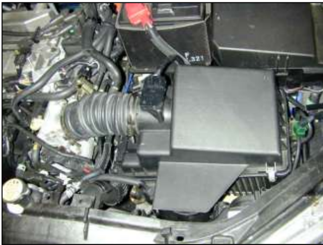
a. Stock air box system installed.
