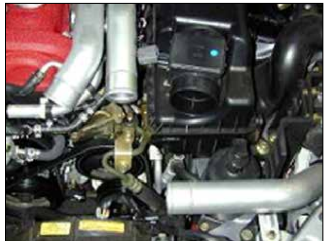
d. Remove the boost pipe elbow and the inlet tube. You will reuse the boost side elbow during the AEM® intake installation.
