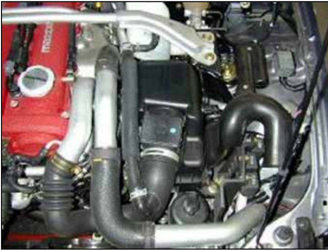
a. Factory air box system installed.
