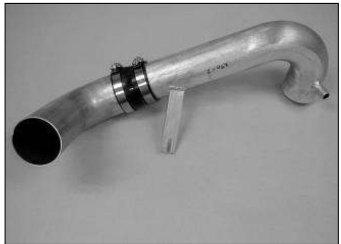
Fig. 9a Intake pipe orientation for Honda Civic Ex models
