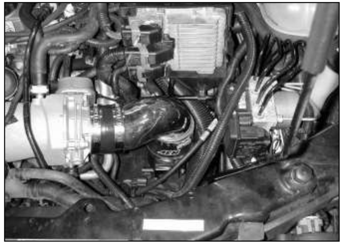
AEM® intake system installed
