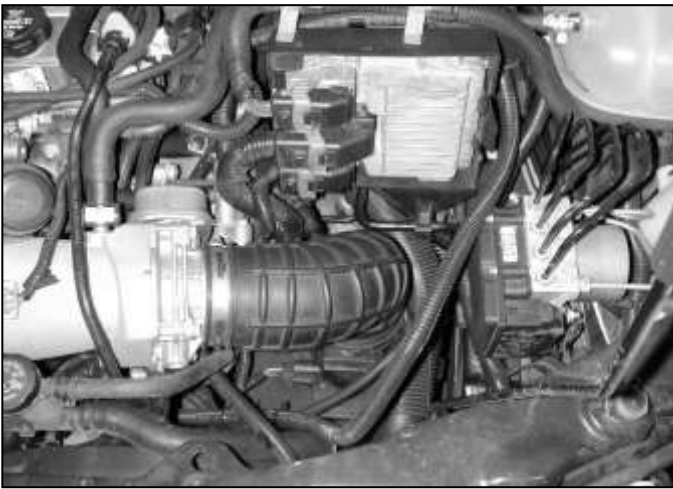
Factory air box system installed
