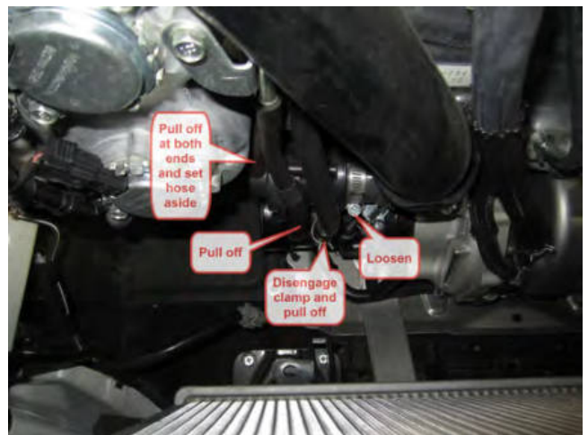
d. Remove the vacuum line to the recirculation valve and set aside (cap steel line with provided cap (Item 9) if desired) as well as the other two lines shown above and loosen the clamp between the valve and the factory charge pipe enough for the clamp to move freely.
