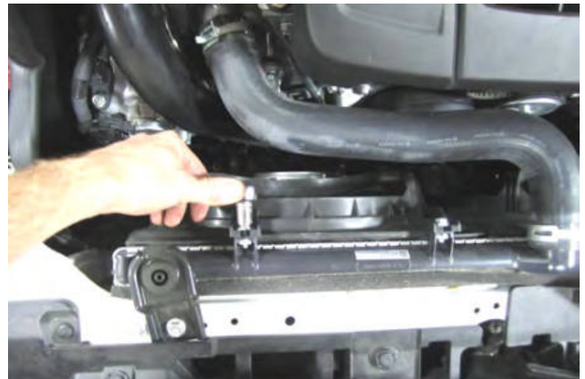
b. Remove fan using a 10mm socket as shown. Once the two top bolts are removed and the power harness at the bottom is disconnected, the fan can be lifted out of the engine compartment and set aside.
