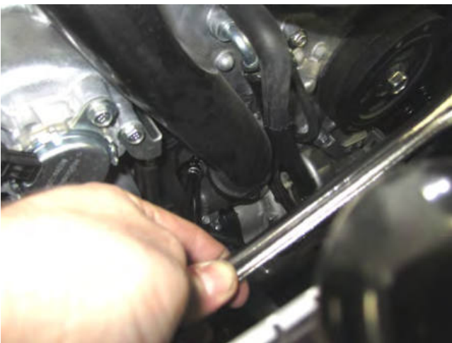
c. Use the 12mm socket with a U-joint and extension to remove the bolts securing the charge pipe flange to the turbocharger.
