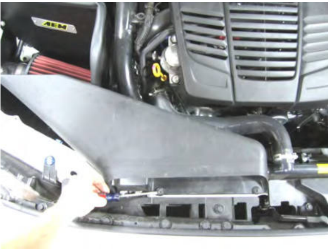
a. Remove factory fresh air inlet duct
