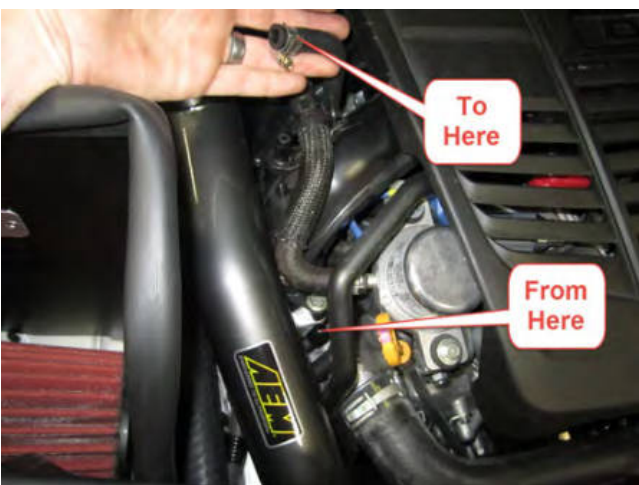
f. Re-route vacuum line through the intake manifold as shown above. Use the other included cap to protect the exposed steel line if desired.
