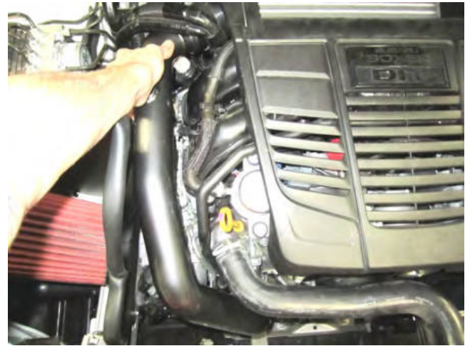
d. Lower your new AEM charge pipe into position and install beginning with the top end at the intercooler and slide lower end into position to install the other flange
