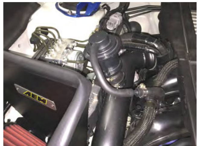
g. Using hose removed in step 2d and connector (Item 10), install your valve and assemble the vacuum supply line as shown.
