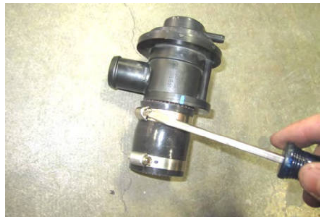
e. Loosely install the smaller coupler and clamps onto your valve of choice (factory valve shown).
