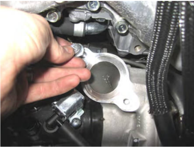
c. Install one of the bolts removed in step 2c loosely into the top-rear flange location on the turbocharger.
