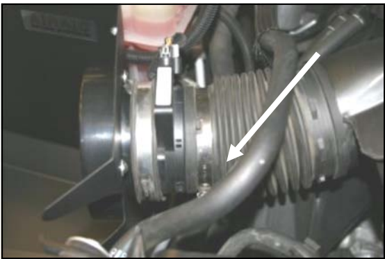
10. Re-connect the factory intake tube to the Mass Air Sensor, and tighten the hose clamp.
