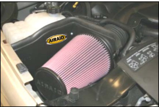
11. Install the Airaid Premium Filter (#1) onto the filter adapter (#4), and tighten the hose clamp. Next install the weather strip (#5) onto the top of the CAD as shown. For ease of installation start at the fender, and work towards the radiator.
