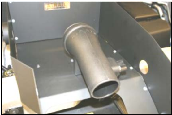
10. Install the Airaid Intake Tube onto the CAD using two 1/4-20 x 1/2" button head bolts (#7) and 1/4" flat washers (#8), threaded up from the bottom of the CAD.
