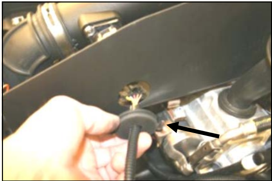
13. Slide the Mass Air Flow sensor connector thru the hole in the side of the CAD, and install the "split" grommet (#16) over the wiring loom as shown.
