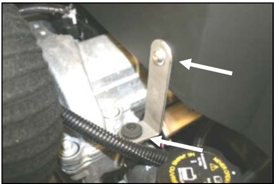
12. Install the small factory grommet removed in step #5 into the supplied bracket (#14). Next slip the installed grommet over the stud on the front of the engine, and bolt the bracket to the CAD using one 1/4-20x 1/2" button head bolt (#7), 1/4" flat washer (#8), and 1/4" serrated nut (#9).
