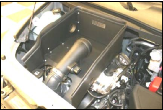
11. Install the assembled CAD into the vehicle by lowering the front into the vehicle first, and then aligning the two grommets on the studs at the rear of the engine. Push down firmly on the rear of the CAD to seat the grommets. Next slide the factory rubber elbow onto the Airaid Intake Tube.
