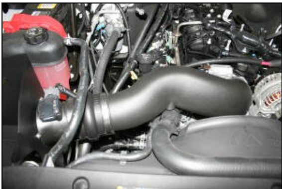
12. Install the Airaid Intake Tube into the hump hose first, and then onto the throttle body. Adjust it for fit, and then tighten all three hose clamps. Reinstall the plastic retainer on the radiator hose into the bottom of the Airaid Intake Tube. Refer to step #3.
