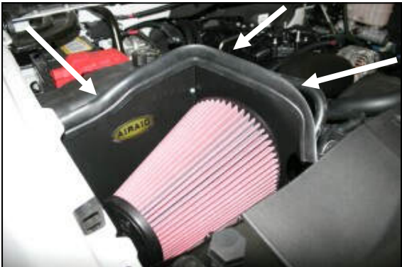
14. Install the Airaid Premium Filter (#1) onto the air filter adapter, and tighten the hose clamp. Next install the provided weather strip (#9) onto the top of the CAD. For ease of install, start at the inner fender, and work your way towards the radiator. Reinstall the beauty cover.
