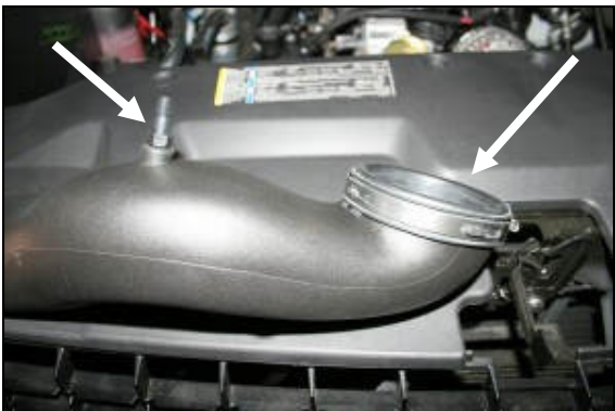
11. Install the 1/4" NPT x 3/8" Barb Fitting (#18) into the Airaid Intake Tube as shown. Next install the supplied coupler and hose clamp (#7) onto the throttle body end of the tube. Leave the clamp loose for now.
