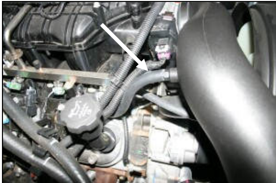
13. Install the 3/8" x 8" breather hose (#8) between the 1/4" NPT x 3/8" barbed fitting in the tube, and the factory port on the valve cover.
