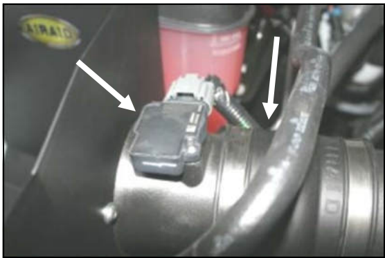
10. Reinstall the MAF sensor onto the filter adapter using two 8-32 x 5/8" Allen Bolts (#13). Do Not Use The Factory Screws! Next install the urethane hump hose (#6) onto the MAF with the two #64 hose clamps (#17). Leave the clamps loose for now.
