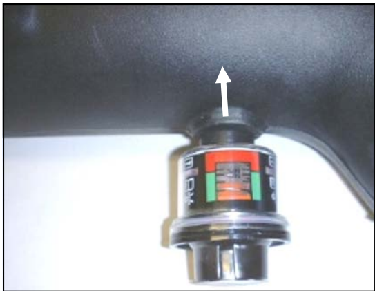
10. Install the factory rubber grommet and air filter minder into the Airaid Intake tube.
