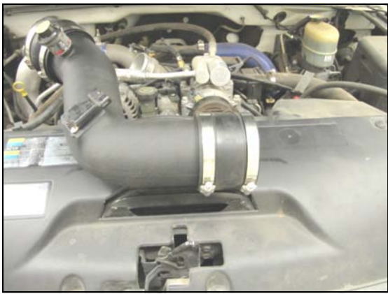
12. Install the urethane coupler (#6) and two #60 hose clamps (#11) onto the small end of the Airaid Intake tube. ( Note: Leave hose clamps loose until final assembly. )
