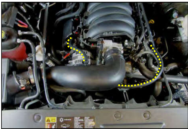
10. Install the Intake Tube and tighten the Clamps. Connect the new breathers to the Barbed Fittings in the Intake tube and the Quick Connect Fittings to the Valve covers .
